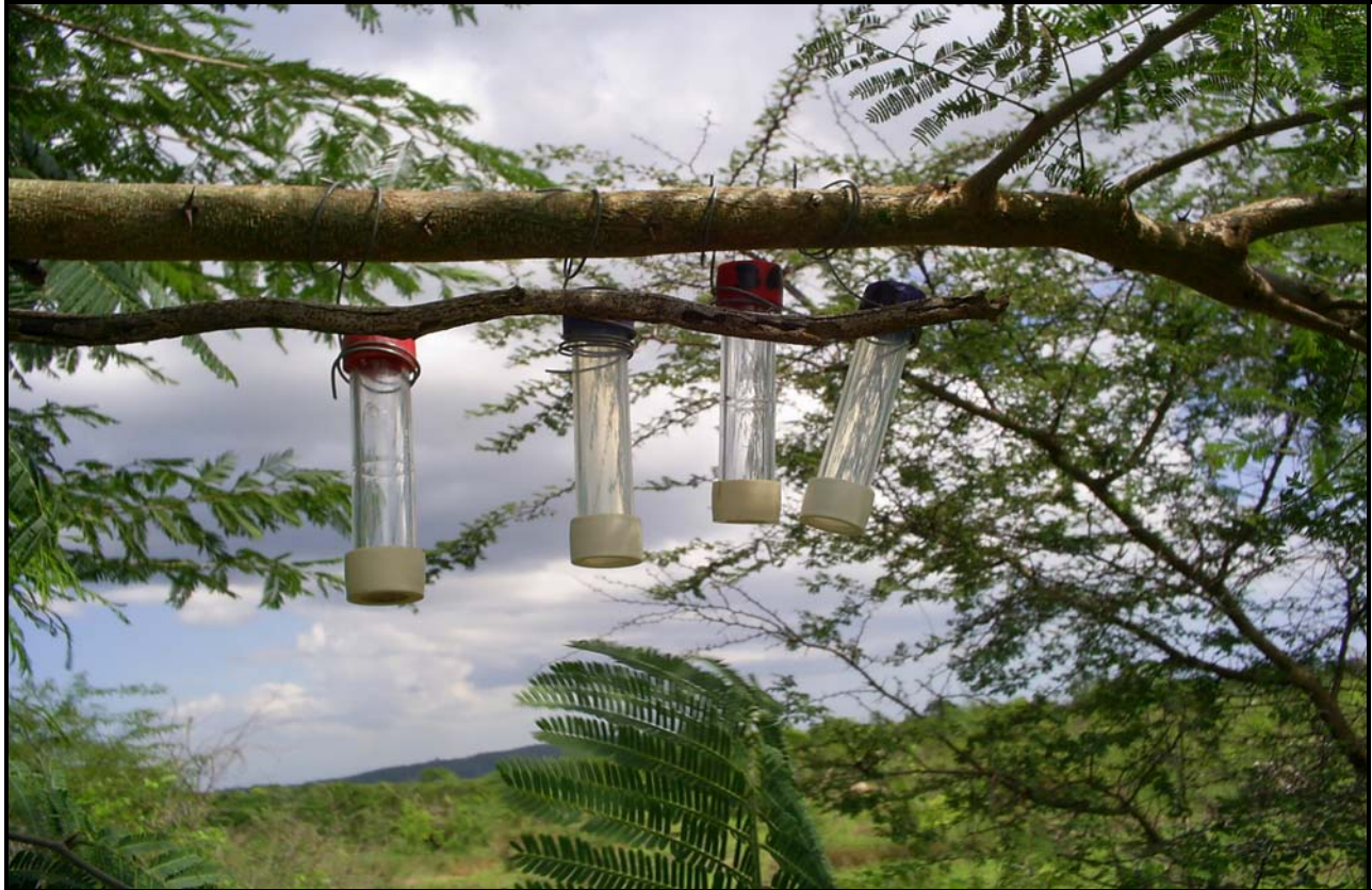
Figure 4: Picture showing the mounted Passive Air Quality Monitors
