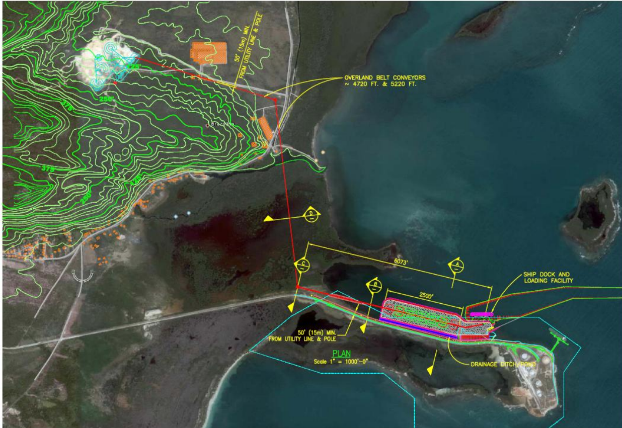
Plate 3-3: Conveyor through Mangroves & Stockpile adjacent Port- Alternative 3
