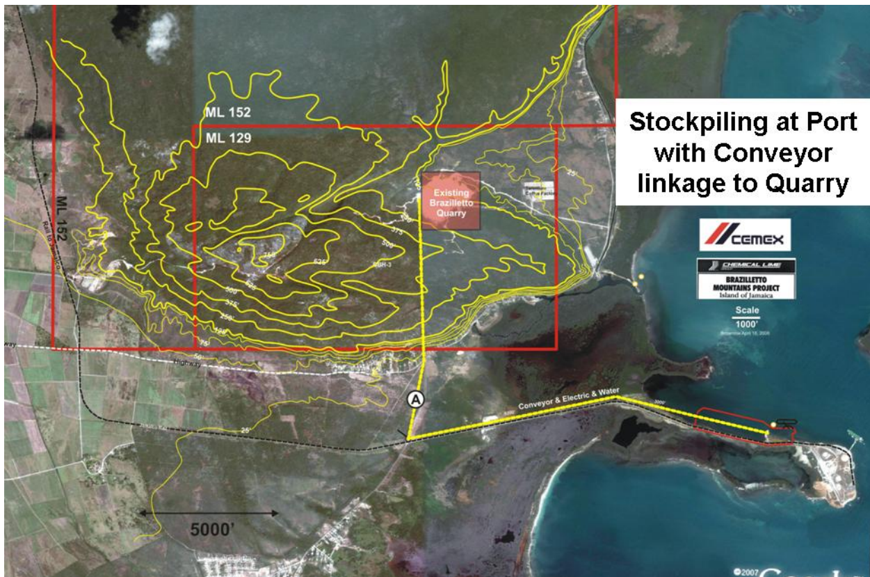
Plate 3-2: Conveyor Corridor & Aggregate Stockpile at Port – Alternative 2
