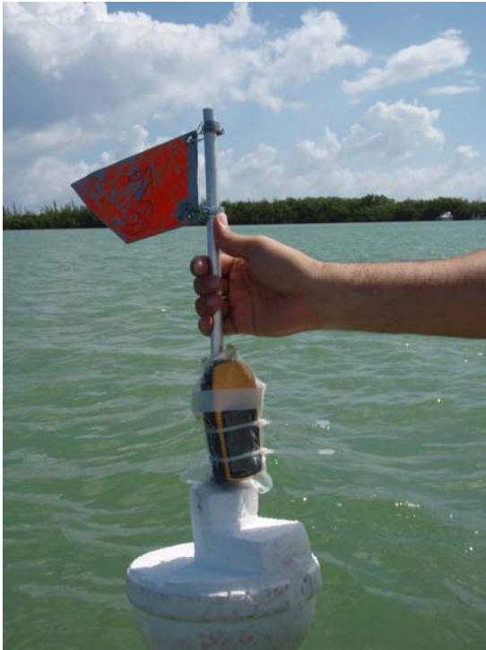
Figure 8 Drogues being deployed in the inner bay
