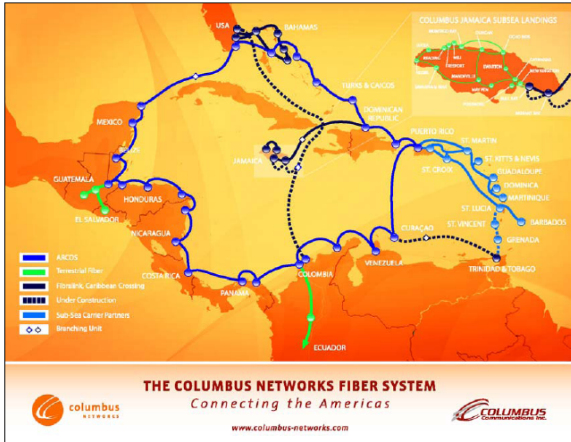
Figure 2-1: Proposed and Existing Regional Fibre-Optic Cable Connections
