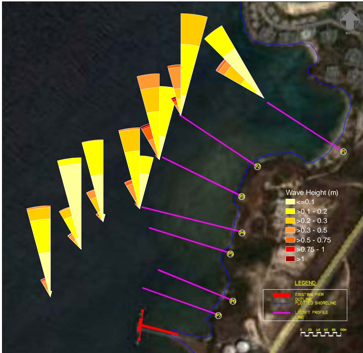
Figure 3.3 Resulting annual wave climate at the location of the selected nearshore nodes
