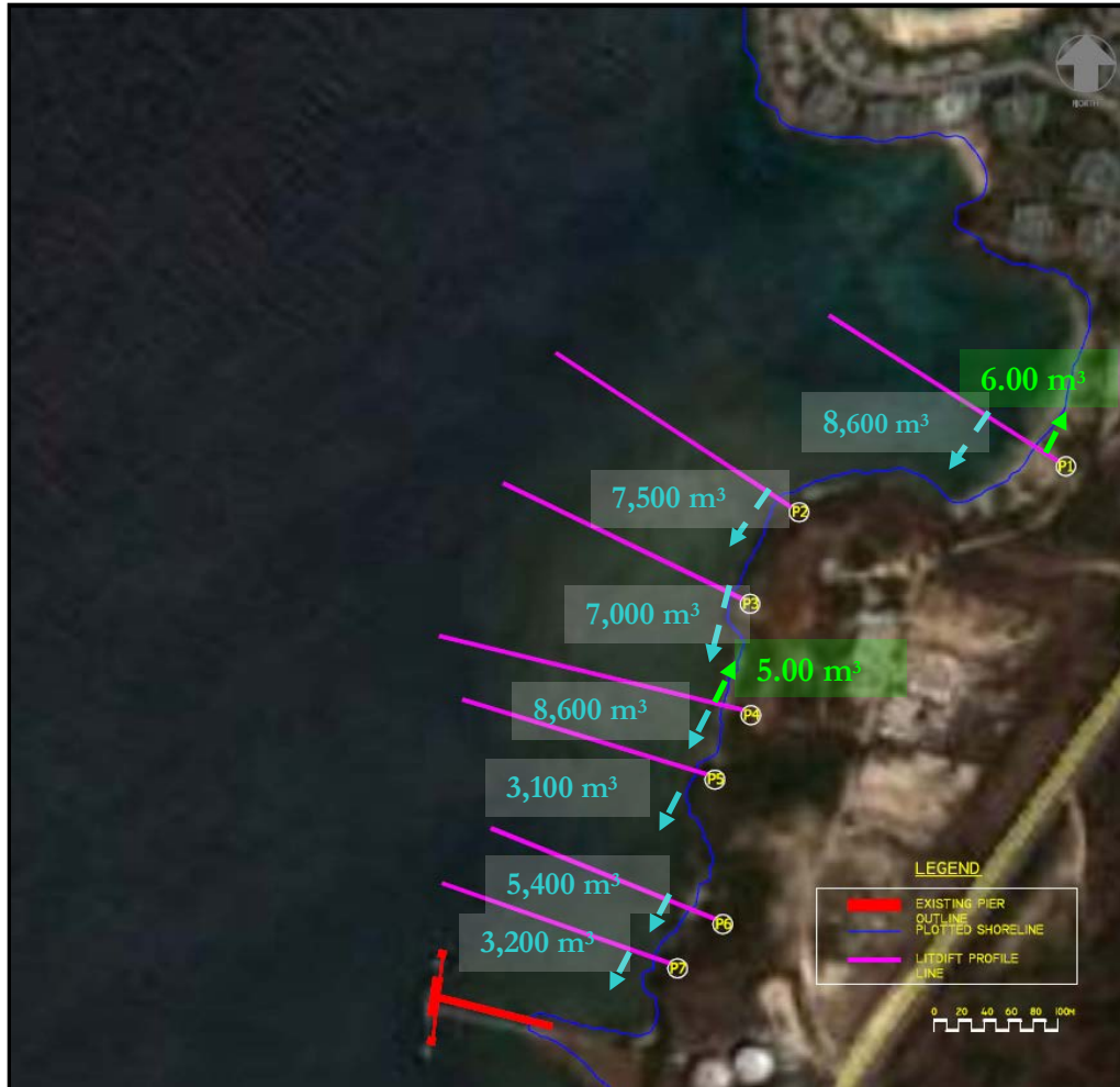
Figure 4.2 Total sediment transport ( m^3 ) accumulated over one year with arrows/values (green/blue) indicating the sediment transport respectively to the north and south
