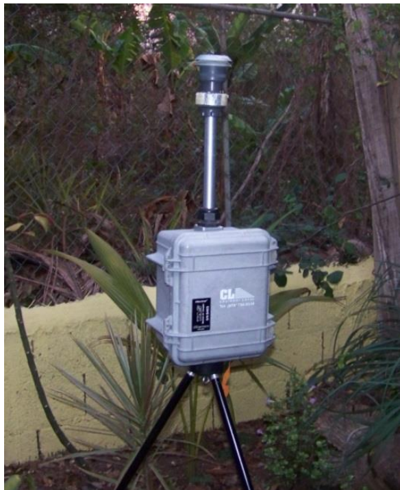
Plate 4-2 Photo showing particulate sampler deployed
