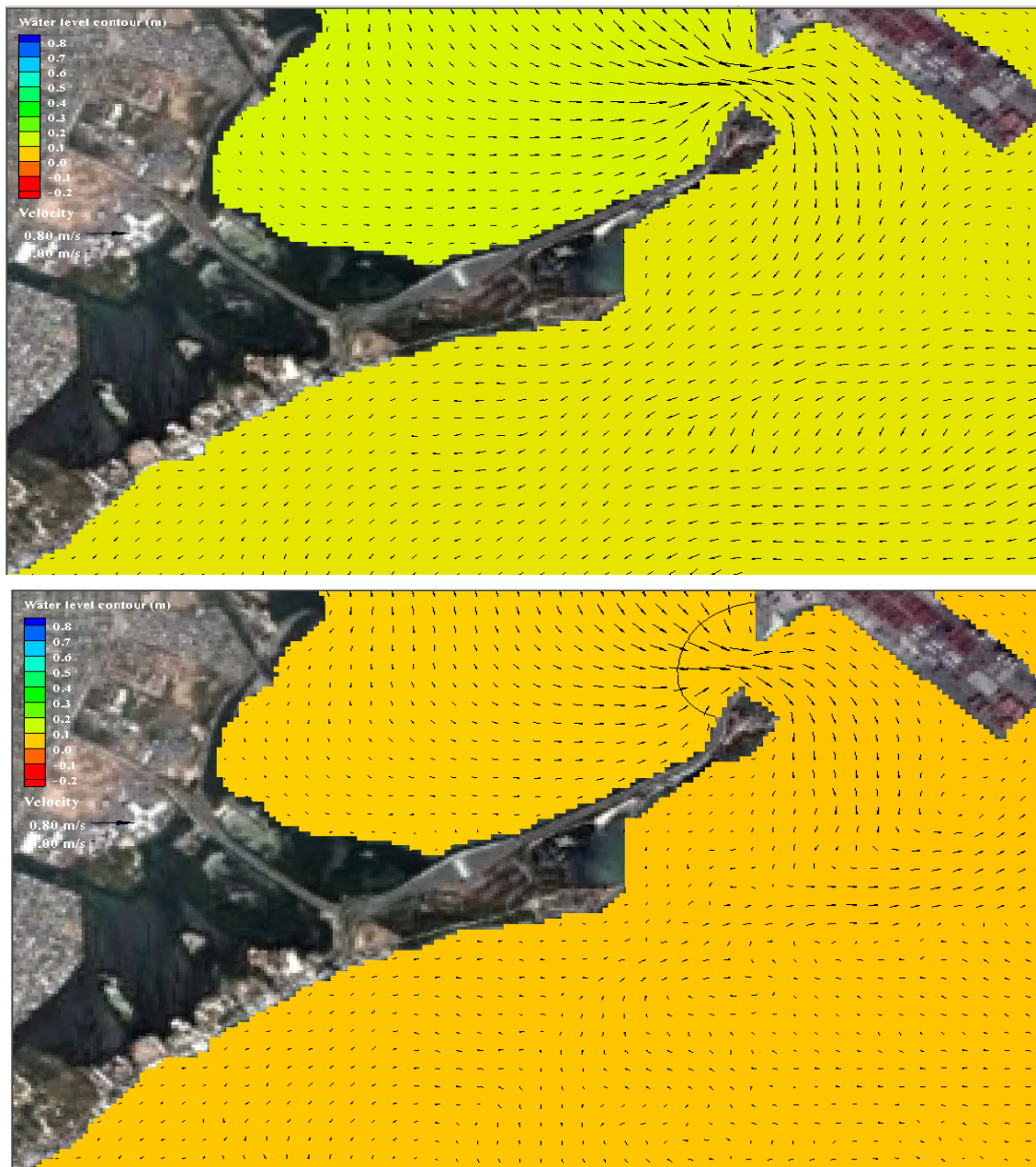
Figure 45: Modelled flow pattern during a spring tide with a large discharge from Hunts Bay. Upper panel: peak ebbing; lower panel: peak flooding. Without the proposed Fort Augusta expansion. NOTE: the vector scale bar equals to 0.8 m/s for both upper and lower panels.
