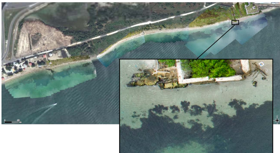
Figure 52: Photo mosaic of surveyed area. The resolution of the mosaic is < 1cm/pixel.
