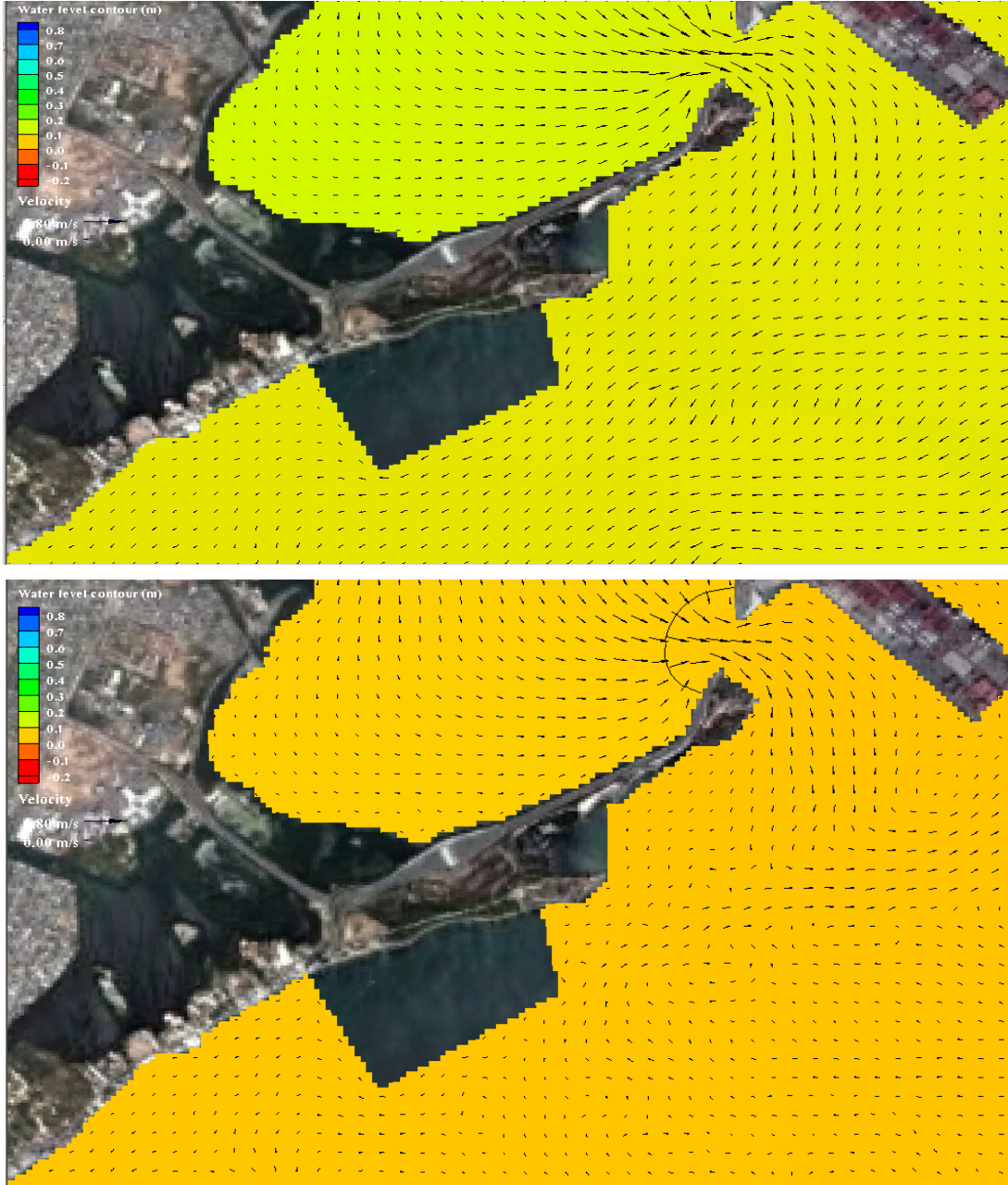
Figure 46: Modelled flow pattern during a spring tide with a large discharge from Hunts Bay. Upper panel: peak ebbing; lower panel: peak flooding. With the proposed Fort Augusta expansion. NOTE: the vector scale bar equals to 0.8 m/s for both upper and lower pane.
