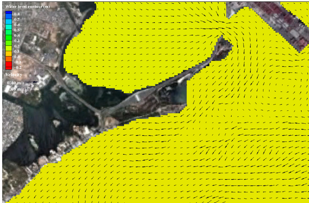
Figure 39: Modelled flow pattern during a spring tide with negligible discharge from Hunts Bay. Upper panel: peak ebbing; lower panel: peak flooding. Without the proposed Fort Augusta expansion. NOTE: the vector scale bar equals to 0.4 m/s.
