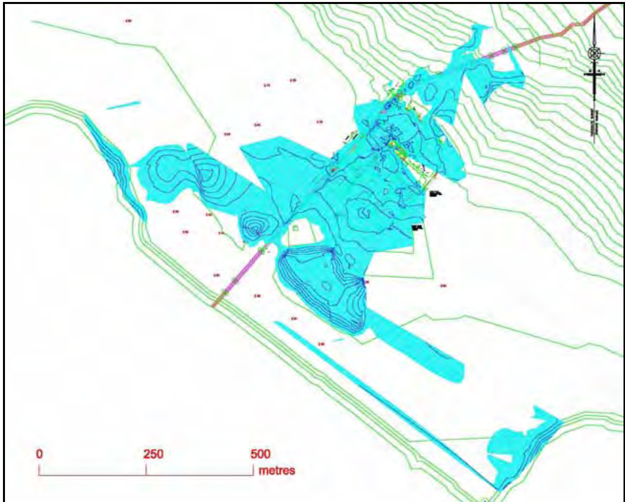
Figure 20 1 in 100 year rainfall event (Blocked Culvert)
