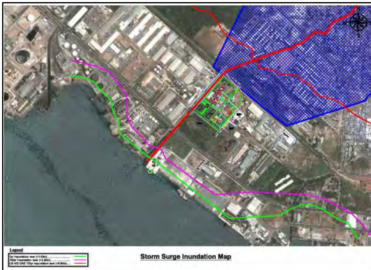
Figure 27 Inundation map showing water surface elevations for the CEAC predicted 50 year and 100 year storm surges as well as the US AID OAS 100 year prediction
