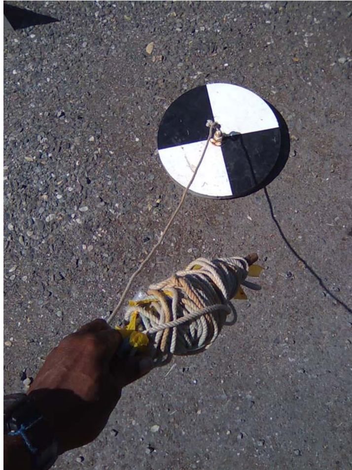
Figure 4: Secchi Disk used for Water Turbidity Measurements at NMIA
