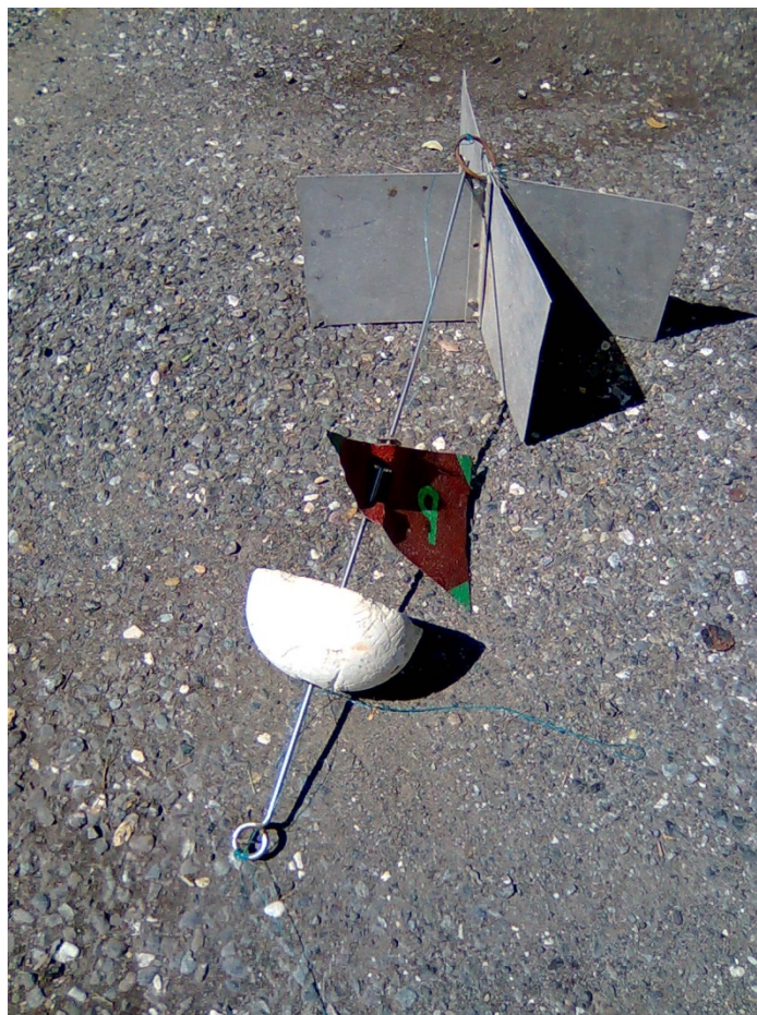
Figure 3: Shallow Water Drogue used for Current Tracking at NMIA
