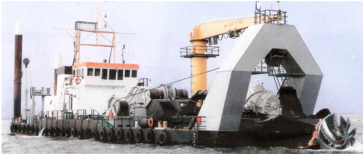
Fig.9 Photo of CSD Mercurius Typical pontoon shallow draught CSD. Most likely this will be the type of machine that will be used for carrying out pump ashore reclamation for the proposed 500m extension of NMIA runway.
