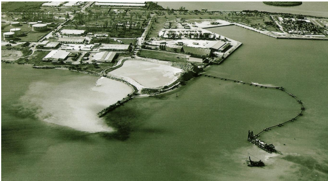
Figure 6.1.2c: Sediment plume from spoil slurry water discharge from spoil disposal area at Montego Freeport Montego Bay during dredging in 1991
