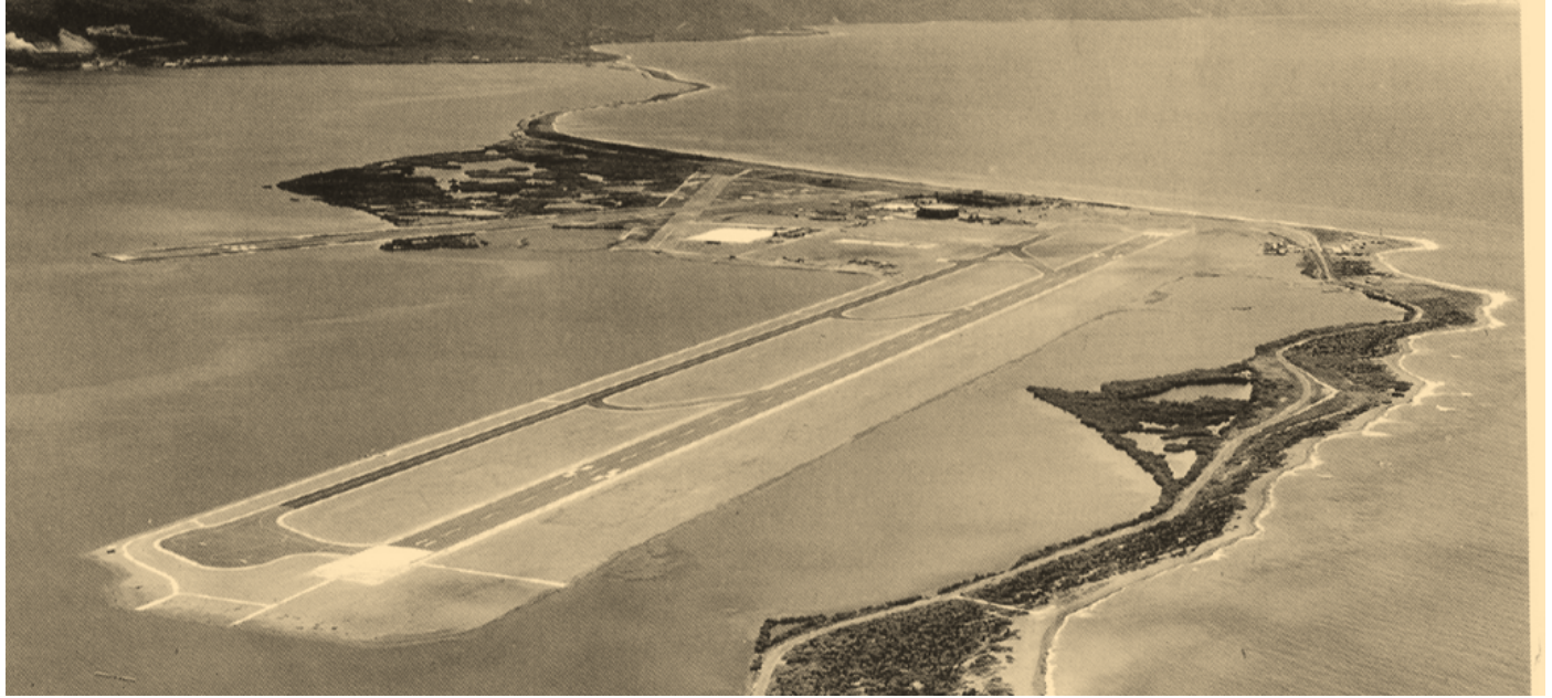
Fig.17 Aerial photo showing the newly completed (August 1959) 1.4 mile long Palisadoes Airport runway
