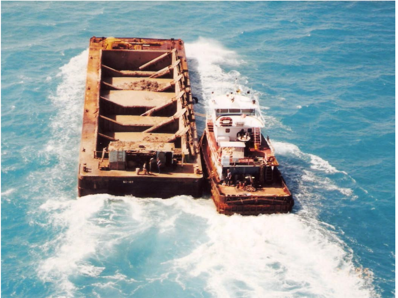
Fig. 11 Photo of a split hull barge being towed away from a dredge site carrying dredged material to be disposed of at a remote dump site. Any Contractor engaged for carrying out this proposed NMIA RESA project will very likely come with equipment such as that shown in the above photo to deal with any off-site disposal situations that might arise.
