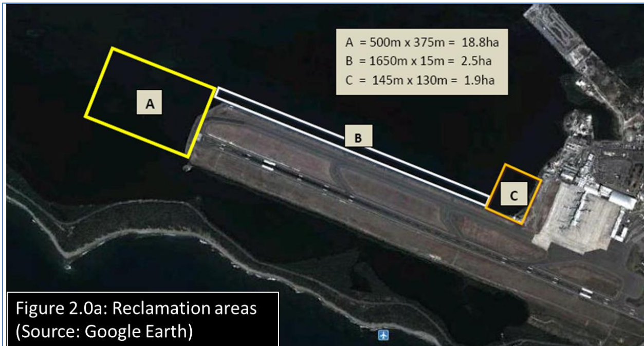
Figure 2.0a: Project site showing areas to be reclaimed. A - This will be the main area for extension of the runway platform; B - This widening of the existing runway platform will allow for better separation between the centerlines of the runway and the taxiway, which presently is somewhat inadequate; C - This reclamation is needed to provide additional land space for aircraft parking and for relocation and upgrading of the airports fire rescue facilities including boathouse. Space will also be provided here for construction of a new electrical substation.
