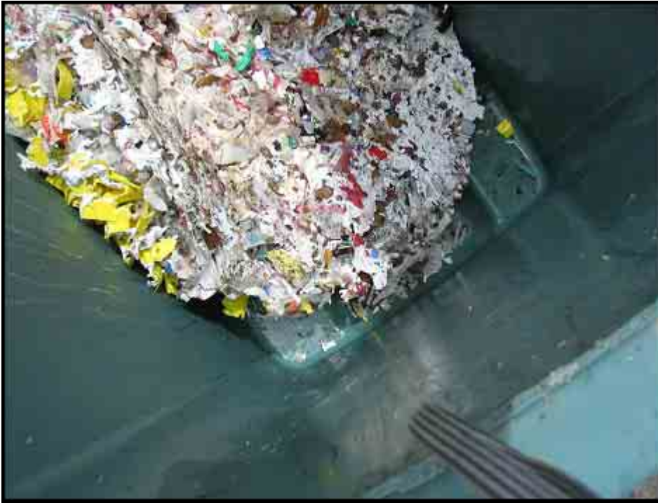
Plate 3.2 Photograph showing sterile unrecognizable waste residue from a T2000 Ecodas Treatment System
