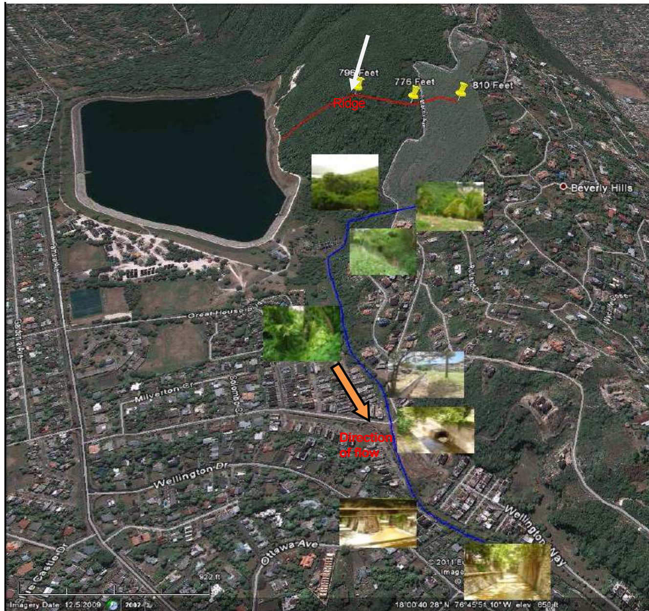
Figure 6.9: Google imagine showing the existing direction of stormwater flows from the proposed Mona Section 1 to the Mountain View Gully
