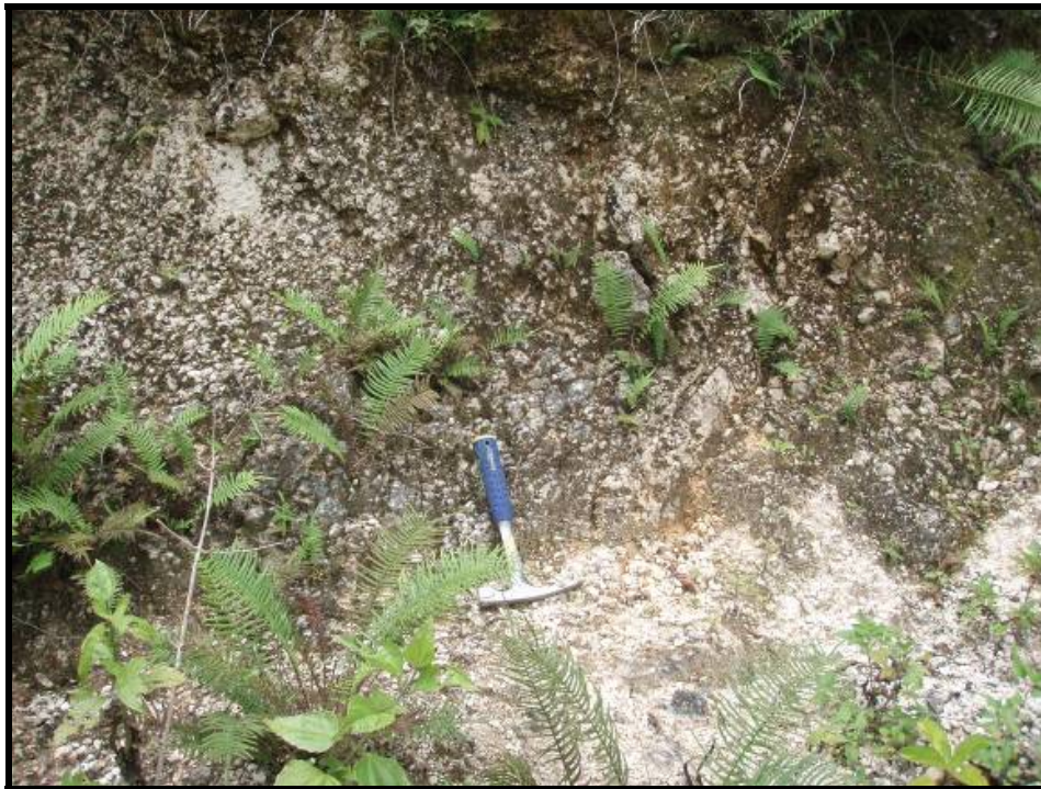
Plate 5-1: Walderston Limestone (exposed on road to Chantilly, north of quarry site, note – rubbly nature)
