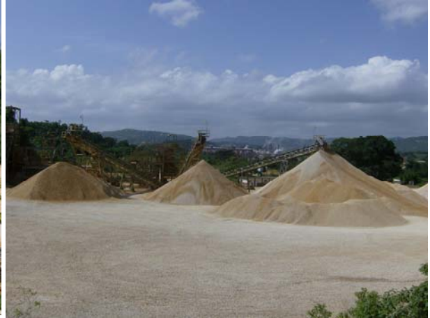
Figure 9-8: Stockpiles and associated conveyor system and crusher in background
