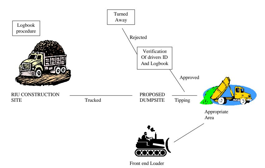
Figure 6 Over simplified flow chart of the disposal of RIU II construction solid waste.
