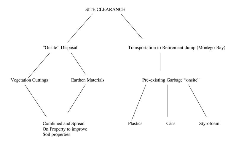
Figure 2 Flow chart of site clearance solid waste disposal at RIU II.
