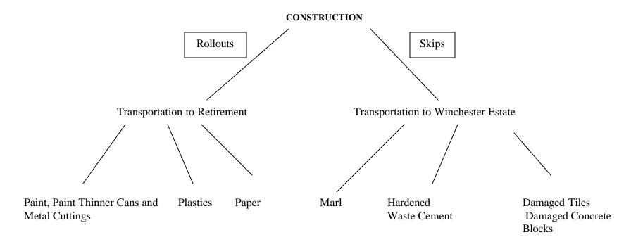
Figure 4 Flow chart of construction solid waste disposal at RIU II.
