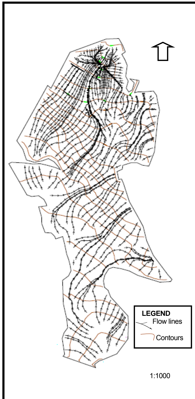
FIGURE SHOWING DIRECTION OF STORM WATER FLOW AT THE SITE OF THE PROPOSED MONA SECTION ONE RESIDENTIAL DEVELOPMENT
