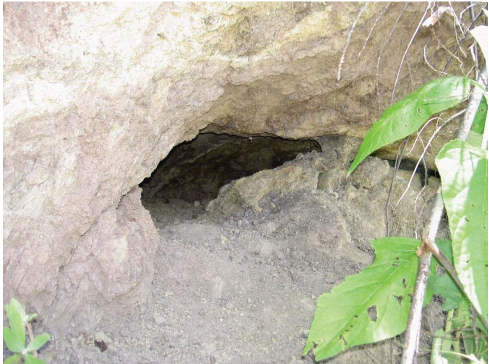
Plate 6.2 Piping in the gypsum deposits near the intersection with the internal quarry road # 2
