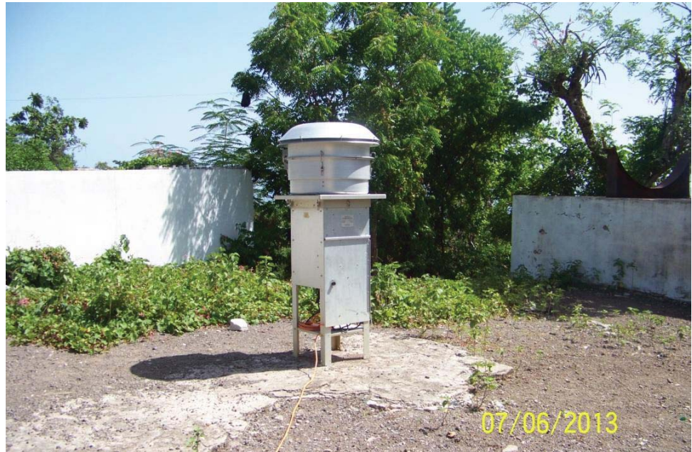
Plate 6.7 Photo showing High Volume sampler at Station P7
