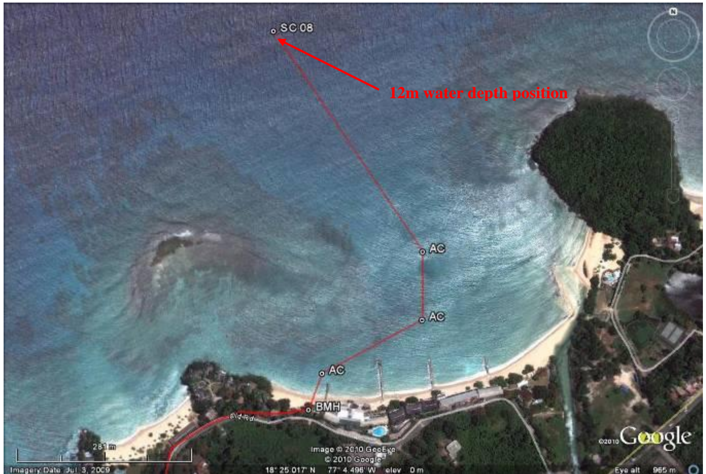
Plate 2-6: Approach to landing point showing reef to be avoided by cable route
