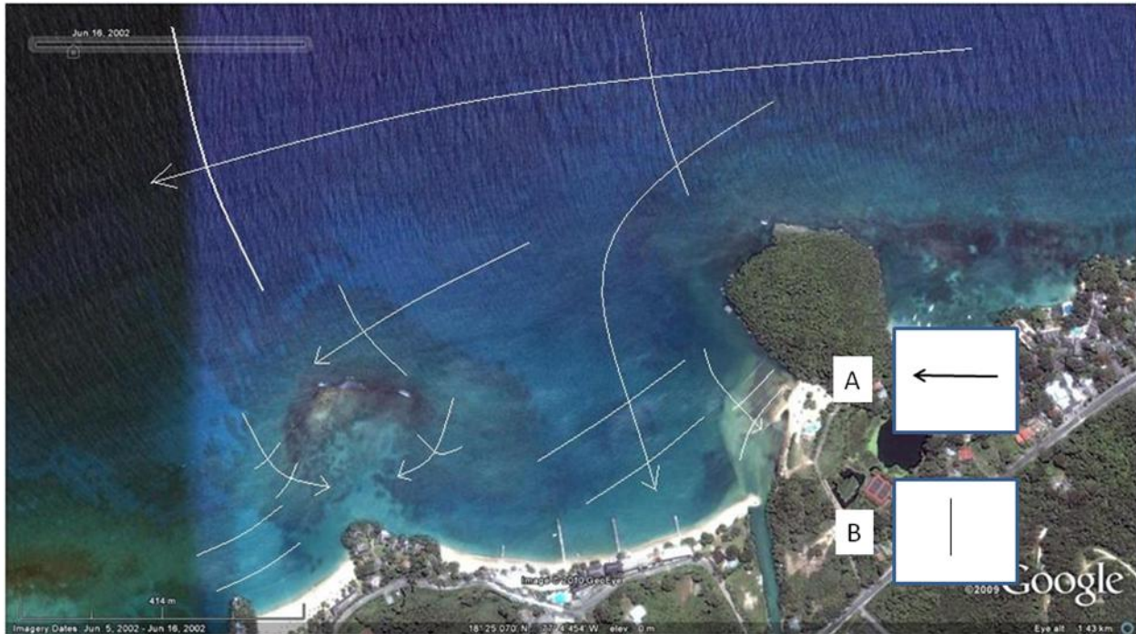
Plate 5-16: Surface Water Movement as Influenced by Prevailing Easterly Winds (A) Orientation of Wave Crests (B) Direction of Wave Movement.
