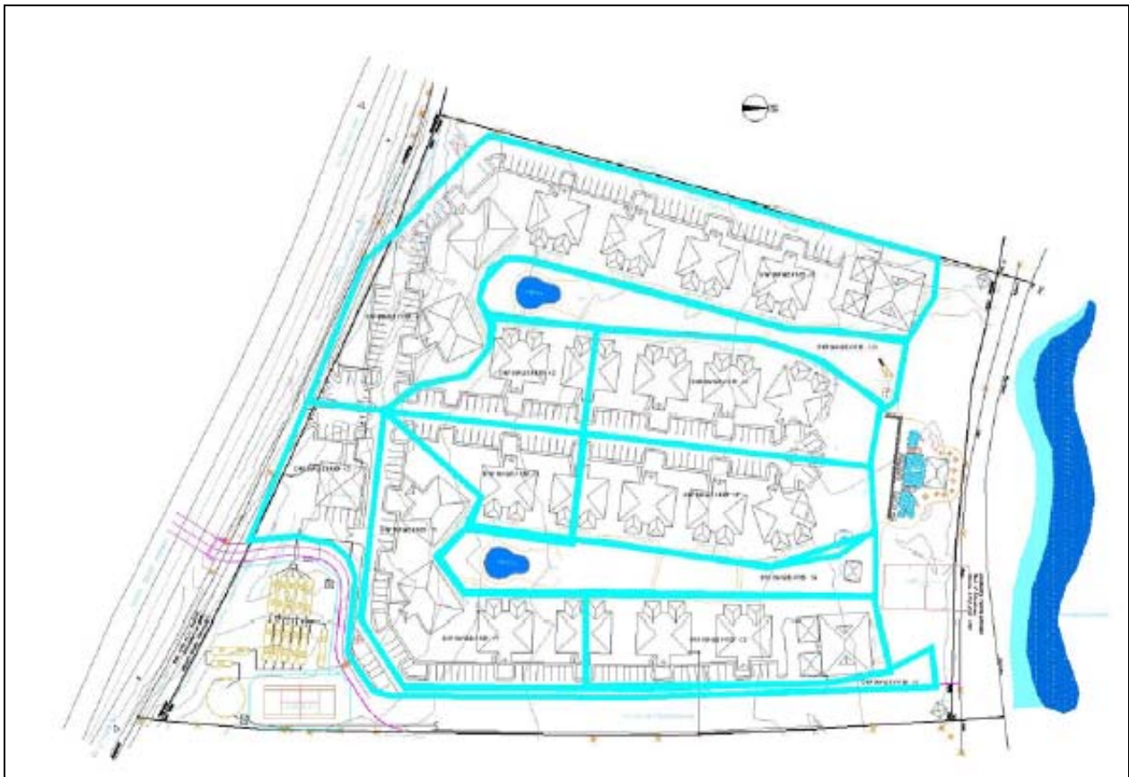
Figure 2 Plan of development showing sub catchments
