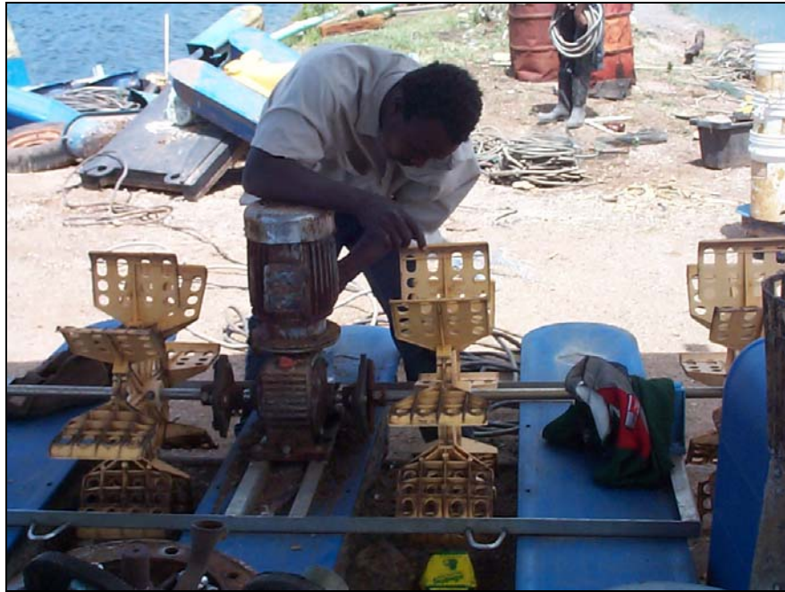
Plate 21. Paddle wheel aerators under repair.
