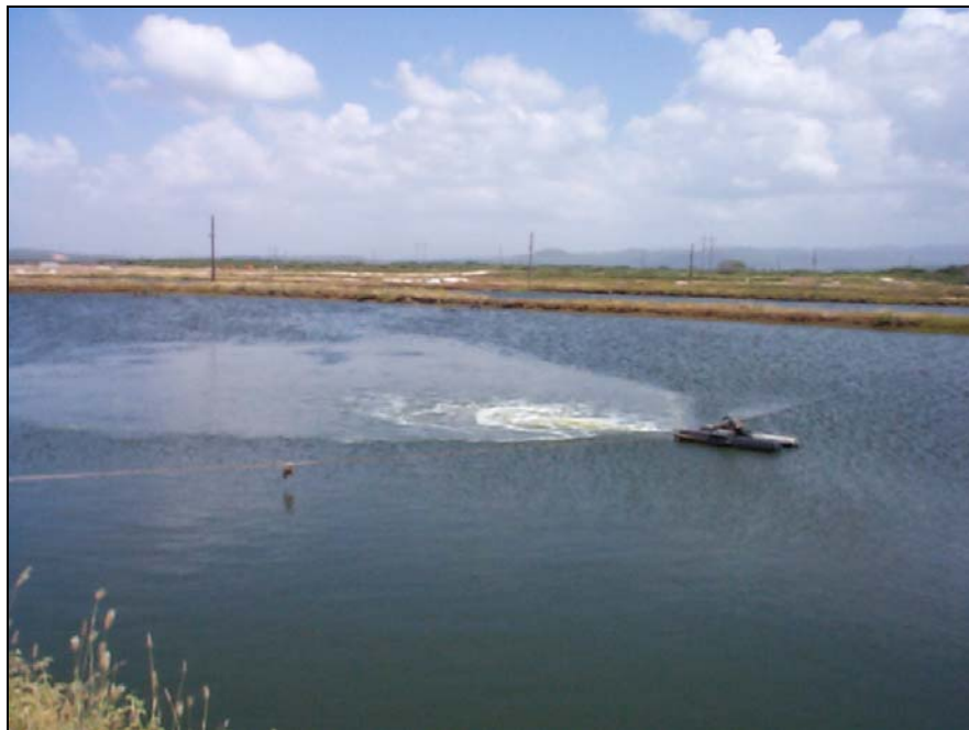
Plate 22. Air injection aerator in shrimp pond.
