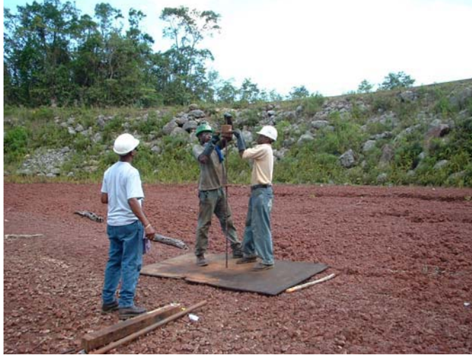
Figure 2: Investigation of the bauxite residue surface using probes
