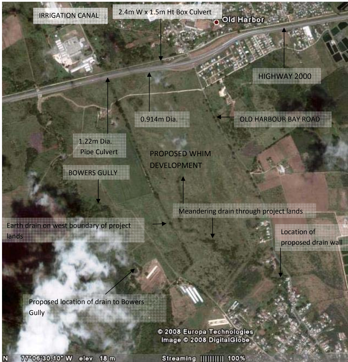
Figure 2 Predevelopment Google Earth image of the proposed Whim development site showing key drainage features
