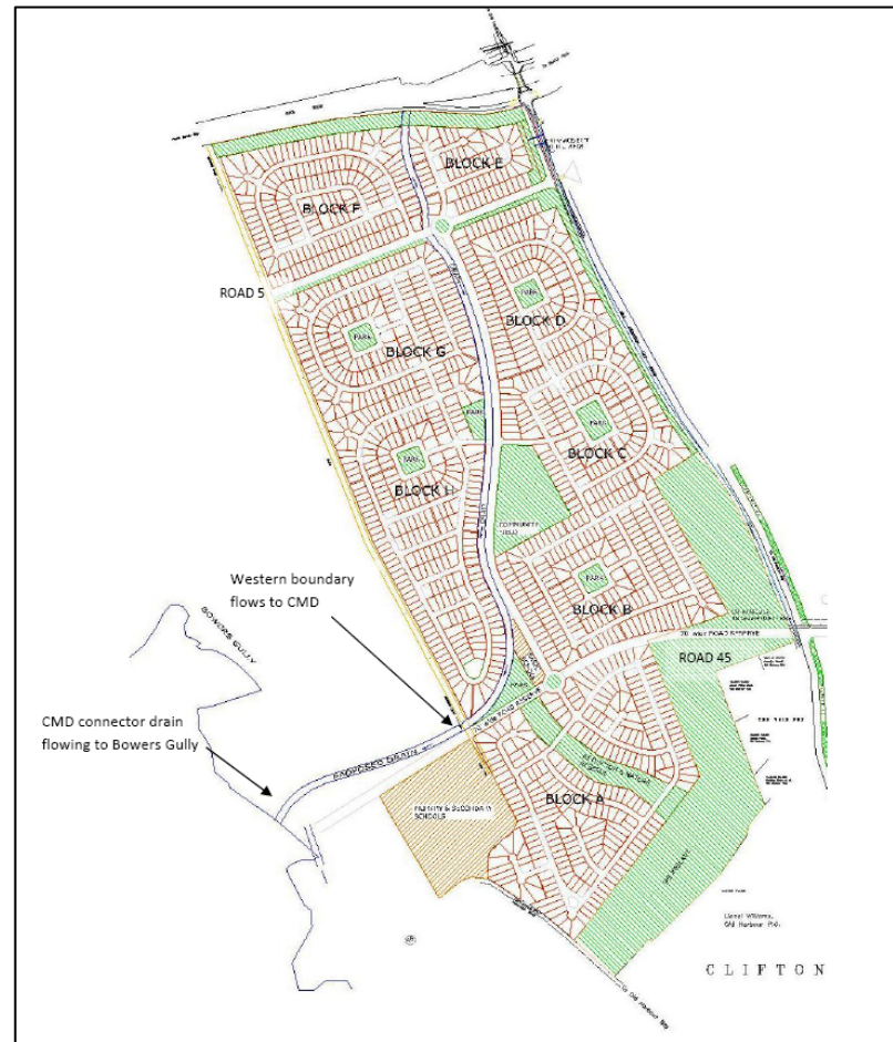
FIGURE 2 - PROPOSED WHIM DEVELOPMENT LAYOUT. BLOCK A WILL DISCHARGE TO THE SOUTH FLOWING OLD HARBOUR MAIN ROAD GULLY. THIS FLOW WILL BE REDUCE BY SOME 75% OVER PRE-DEVELOPMENT FLOWS AND WILL NOT INCREASE THE FLOOD RISK IN THE TOWN.
