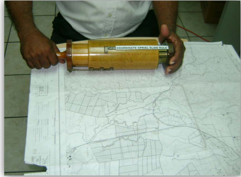
Measuring using Coordinate spiral slide rule
