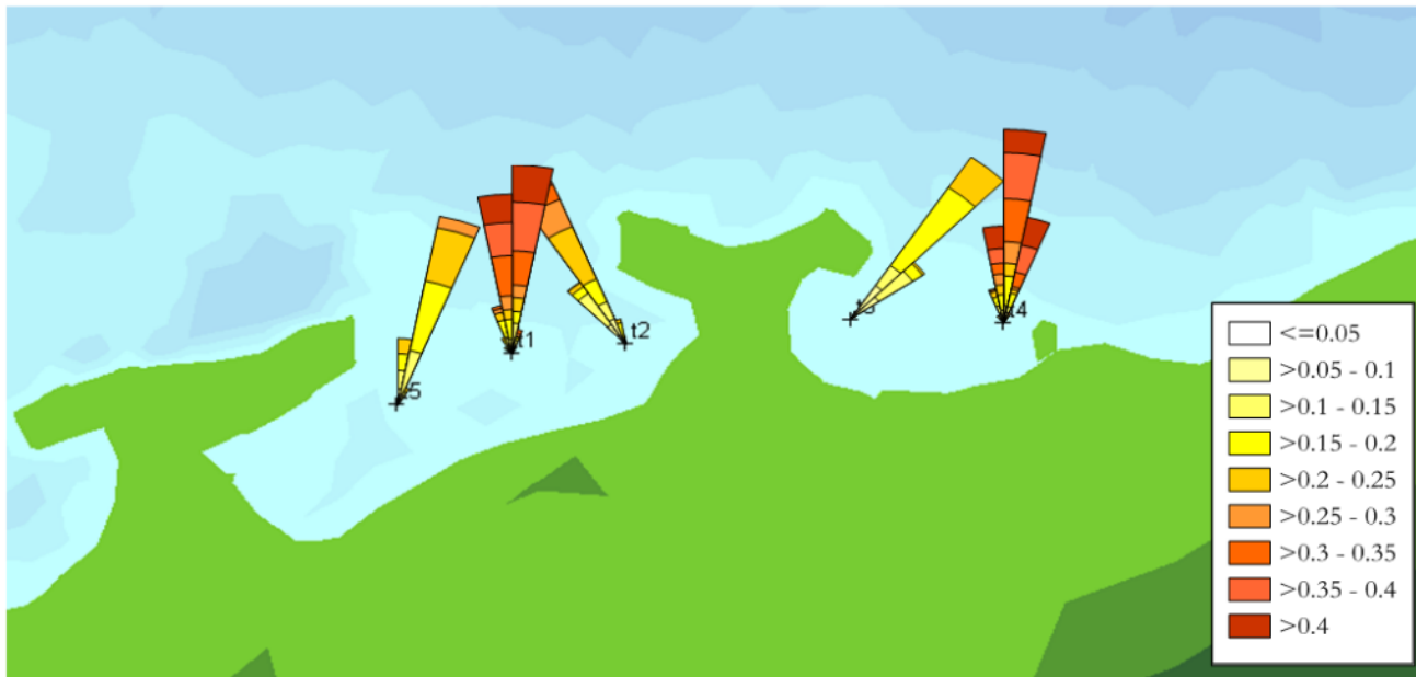
Figure 3.4 Wave Rose plots of typical conditions (binned operational waves) at the site
