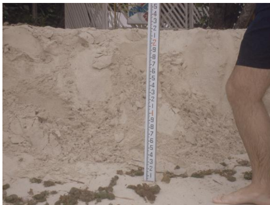
Figure 7. Observed erosion of approximately 0.6m in the southern section of Long Bay .
