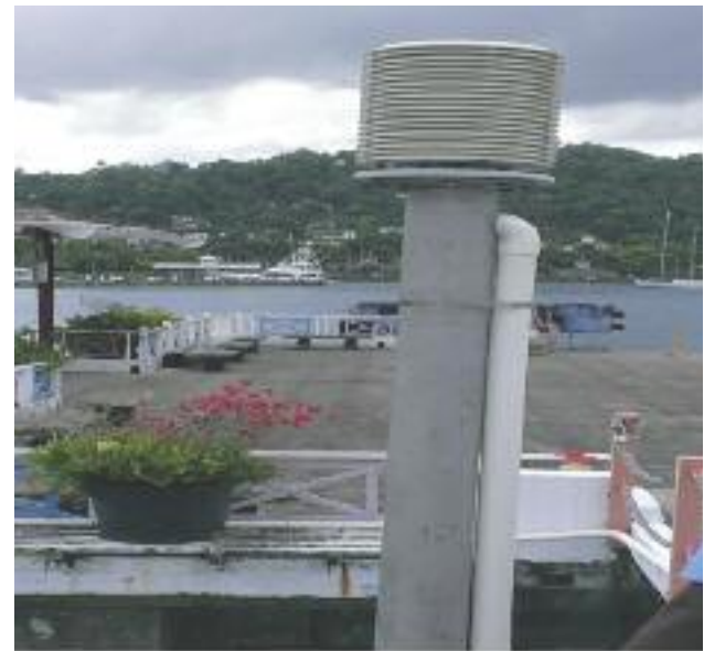
Tide gauge located at Port Antonio Pier.
