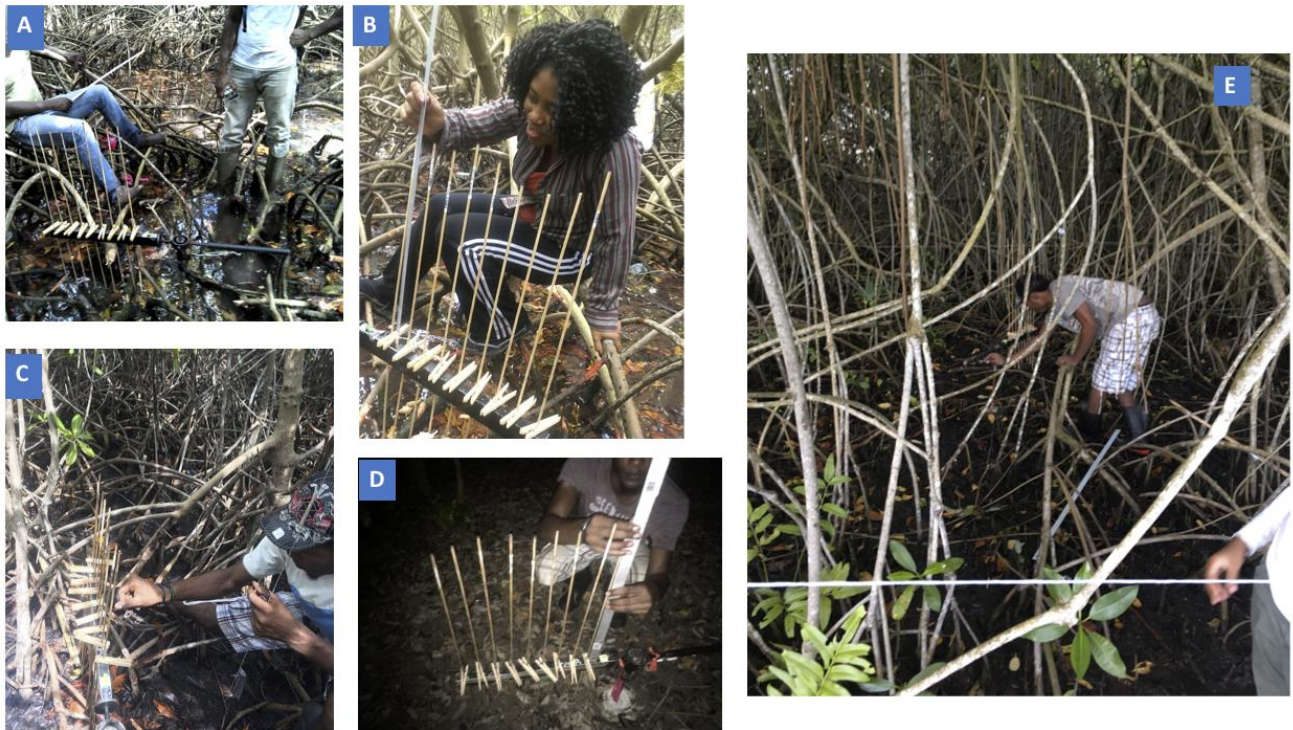
Figure 11: Elevation measurements are being taken with a RSET removable device. A: Set up at Plot 1 Freeport, St. James, B: Measurement at freeport plot 1, C: Measurement at Portland Cottage site 2, D: Measurement at Rodney Street Site, E: Measurement at Bogue Road site.
