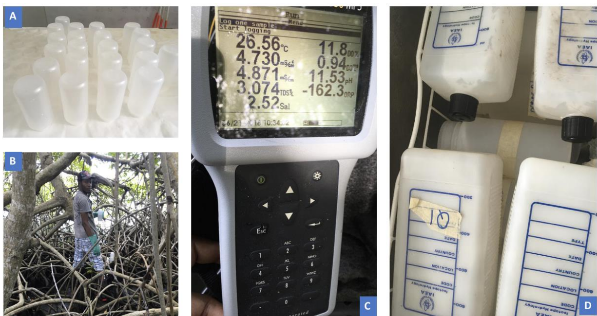
Figure 14: Evaluating the physical parameters of the water within mangrove systems. A: acid-washed HDPE bottles left to dry prior to field day, B: Water is collected along a transect at each site, depending on the water level along the transect, it may take multiple tries to fill bottles, C: YSI collected in-situ water parameters, the data and time is recorded along with corresponding GPS coordinates, D: Sample bottles are labelled and stored according to protocol for analysis.
