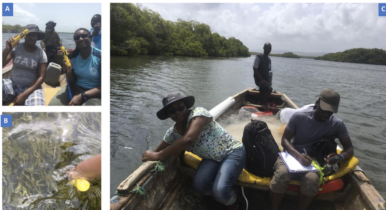
Figure 15: Use of depth sounders along with GPS to collect bathymetry data. A: Hondex digital depth sounder devices are shown. B: device should be emerged in water and held vertically to collect depth readings, C: two depth readings are collected simultaneously along with GPS coordinates.
