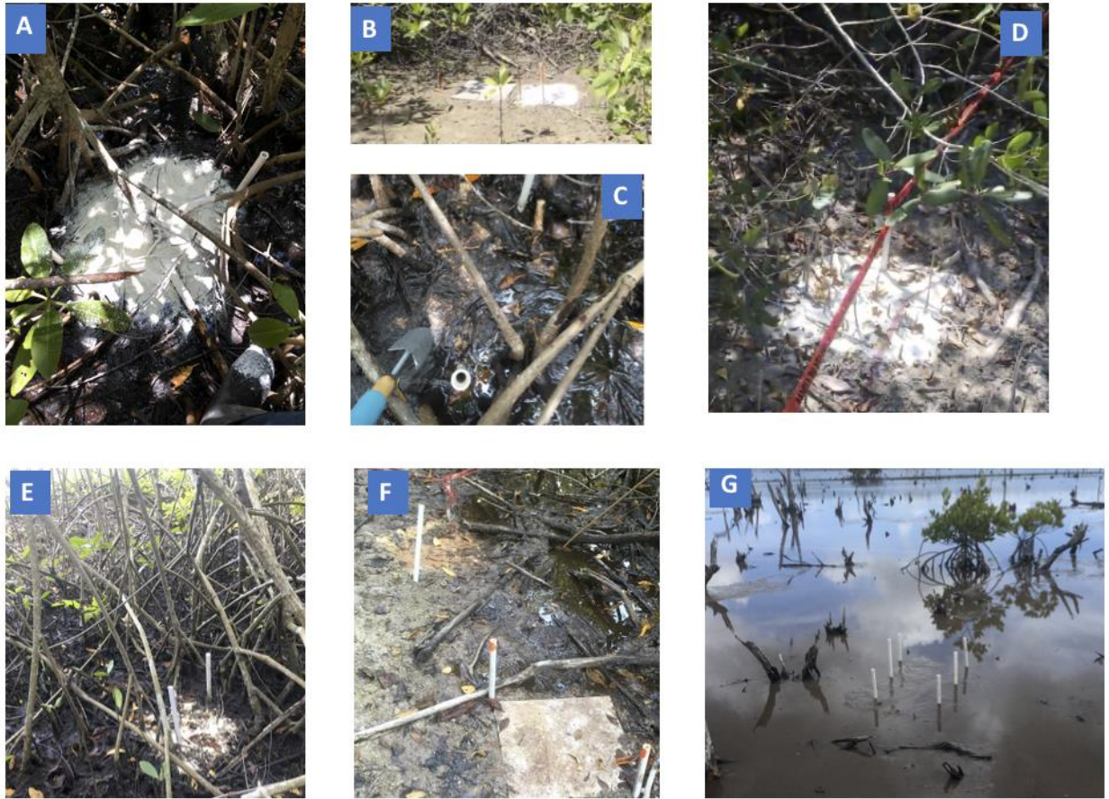
Figure 10: Different views and setting of installed horizon marker and sediment plate (tile) for accretion or erosion records. A: Horizon marker being laid down at Portland Cottage site 2, it is important to dust off roots so the horizon marker is flat. B: Horizon marker at Plot 2 Freeport and adjacent tile, C: Horizon marker covered by a thin layer of sediment, thickness of sediment is being checked with a spade and ruler. D: Horizon marker with no sediment, only sparse leaf litter after a month at Freeport, E: Horizon marker with leaf litter at Bogue Rd, F: Horizon marker and Sediment tiles with negligible sediment after 2 months. G: Horizon marker eroded in sections at Portland Cottage Site 1.
