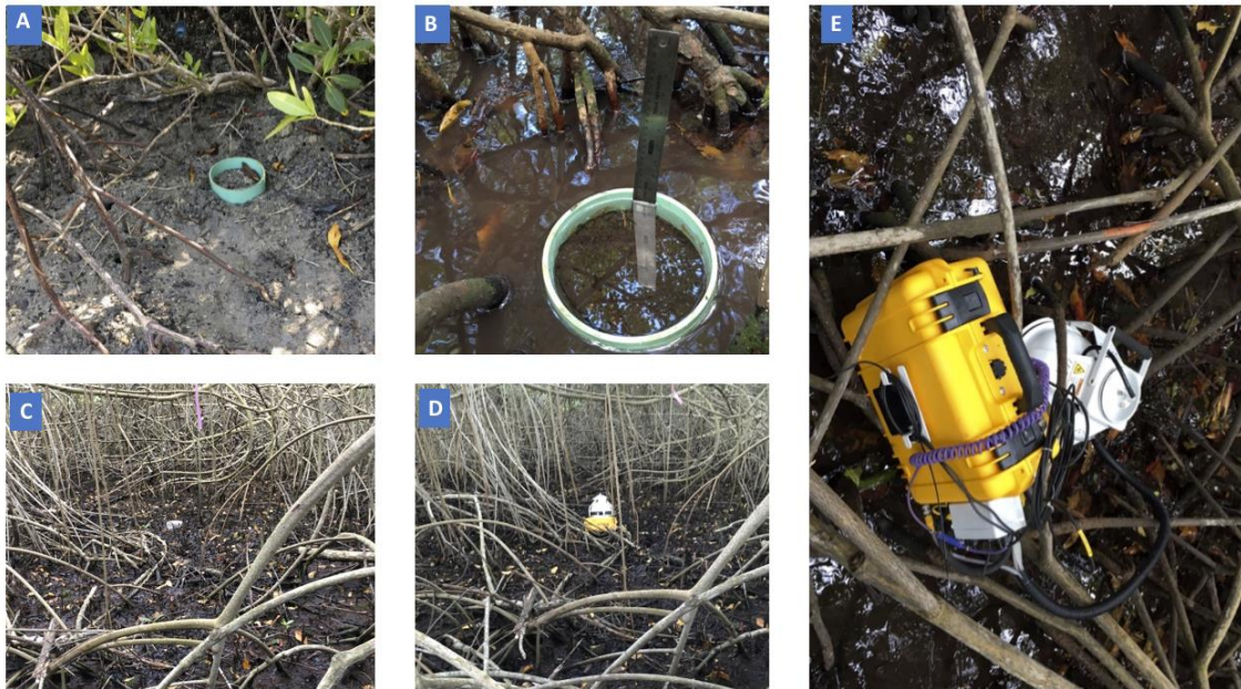
Figure 16: Equipment and process of collecting gas flux data. A: Collar deployed in substrate, B: Collar can be deployed if the substrate is saturated, C: collar deployed and marked with flagging tape along with GPS to facilitate easier relocation and measurements, D and E: Survey chamber mounted to collar and allowed to collect readings for 10 minutes per collar after equilibration period of 2 h has elapsed.
