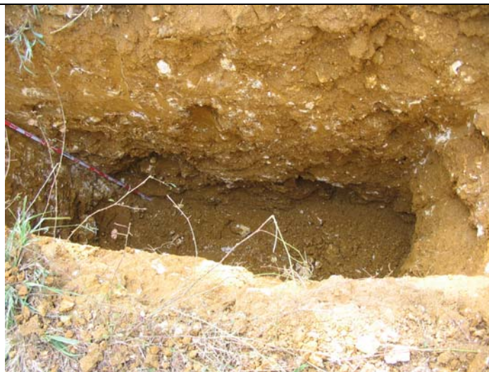
Figure A.12: Pit 6 completed on hard cobbly layer
