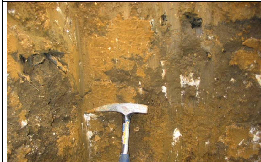
Figure A.9: Pit 4 former land surface at 1200 mm, darker soil and tree roots
