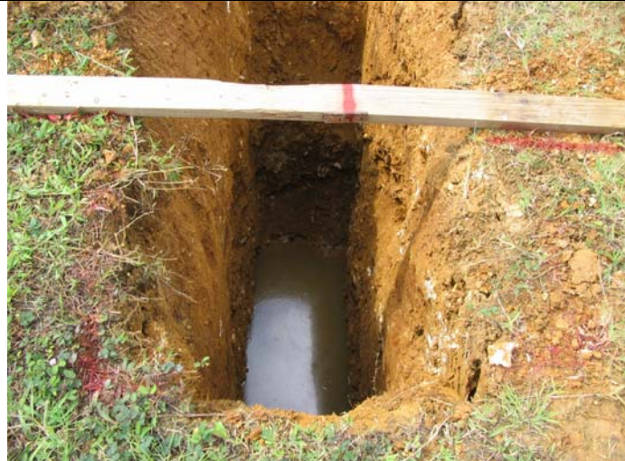
Figure A.7: Pit 3 water immediately after emplacement for percolation test; also shows test measuring point
