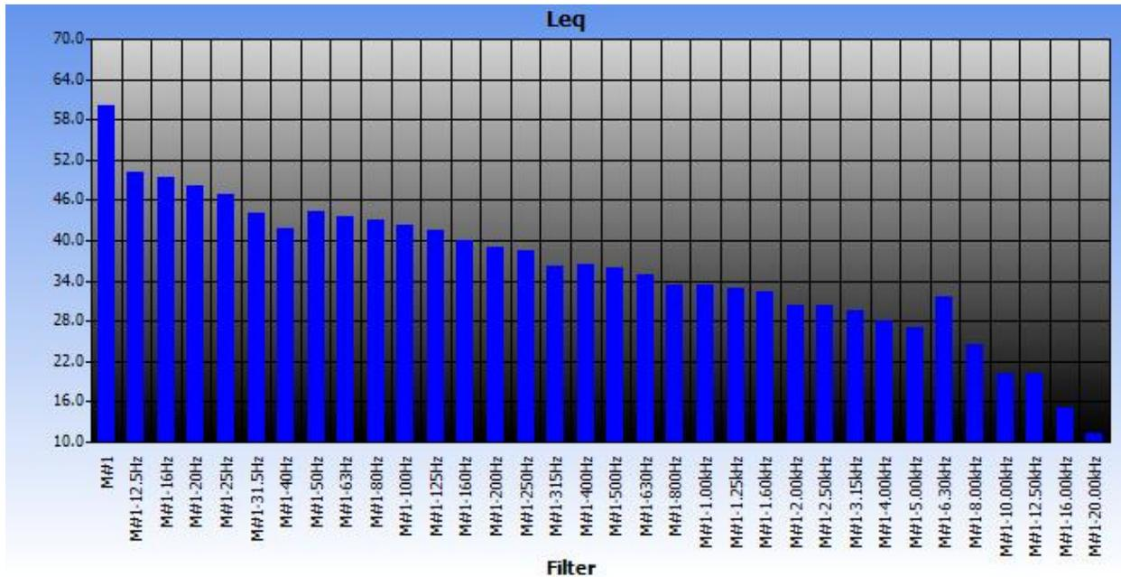
Figure 4-34 Octave band spectrum of noise at Station 4
