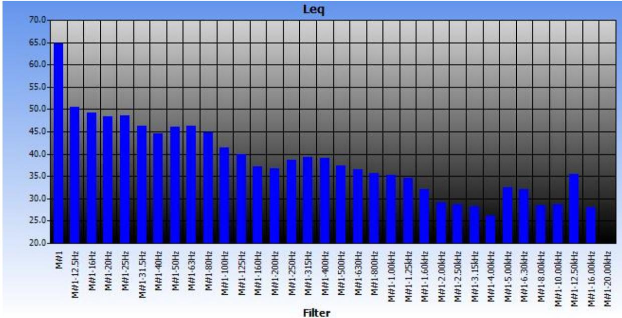
Figure 4-28 Octave band spectrum of noise at Station 1
