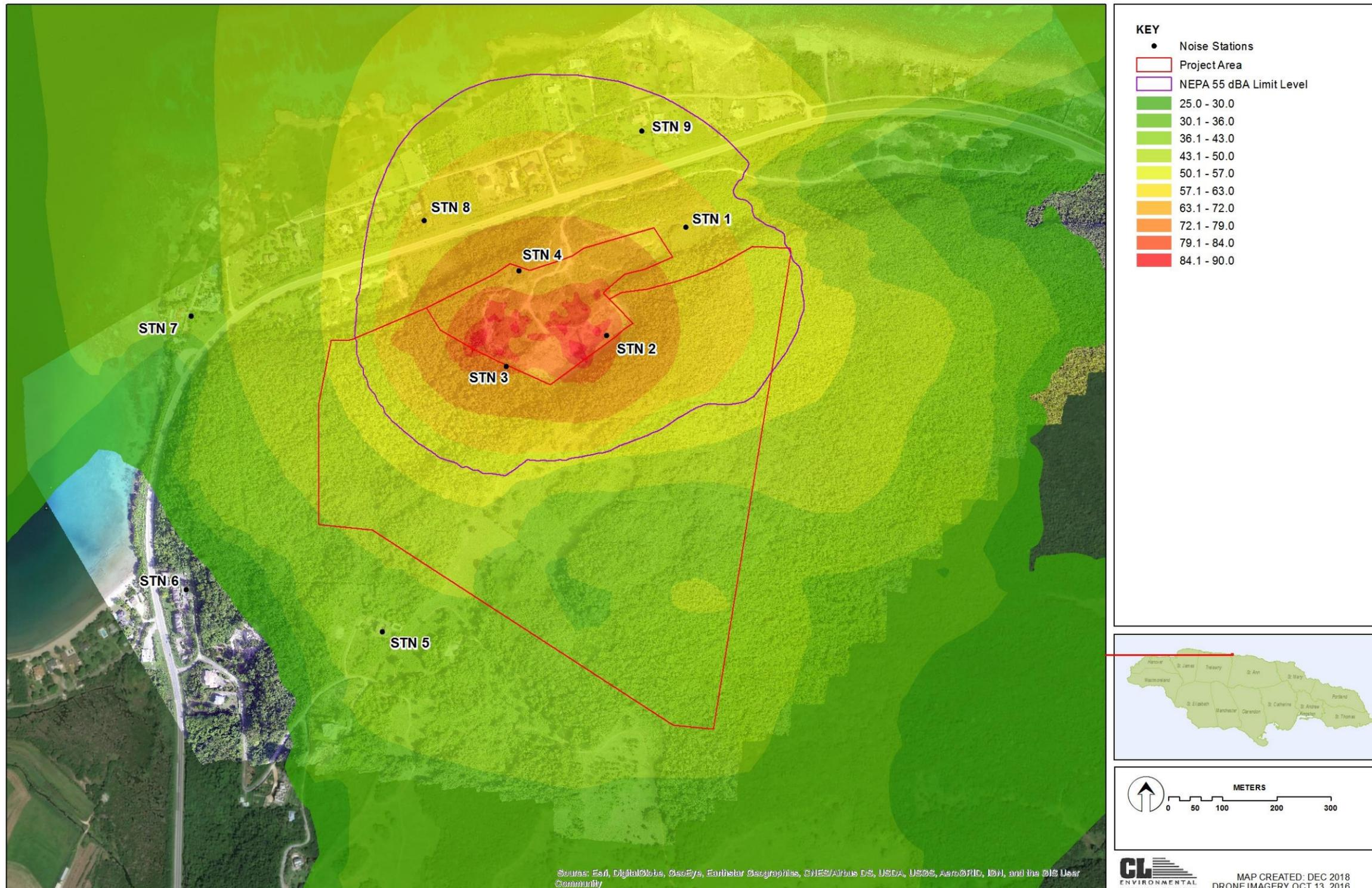
Figure 6-10 Predicted noise emissions from the quarry operations using Concaawe Prediction Method (wind from the southwest)
