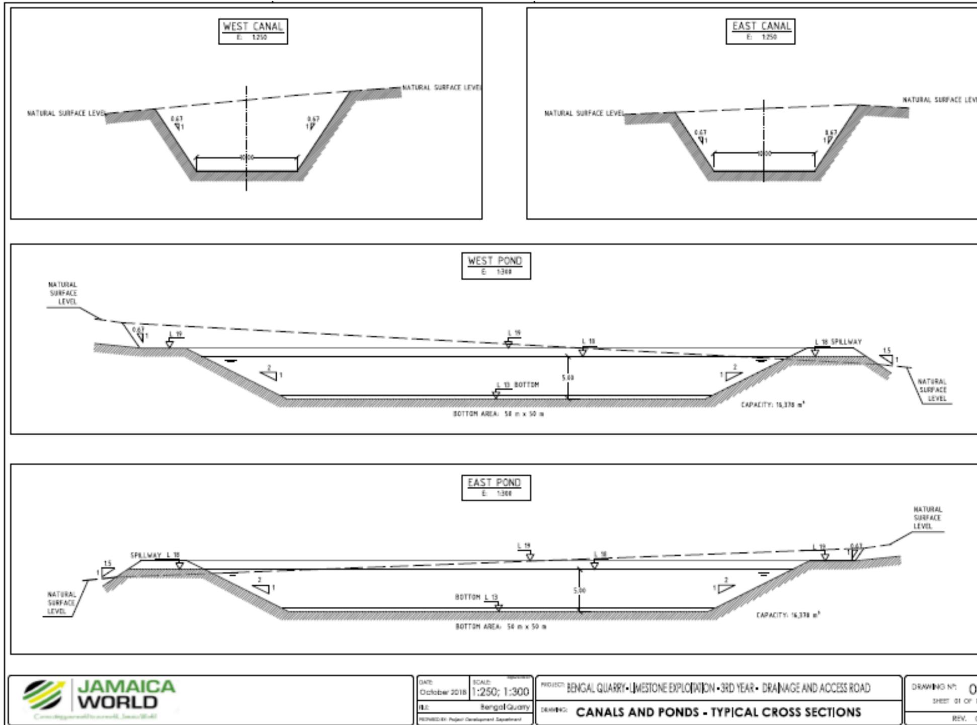
Figure 3-5 Sizes and dimensions of the sedimentation ponds and the drainage canals
