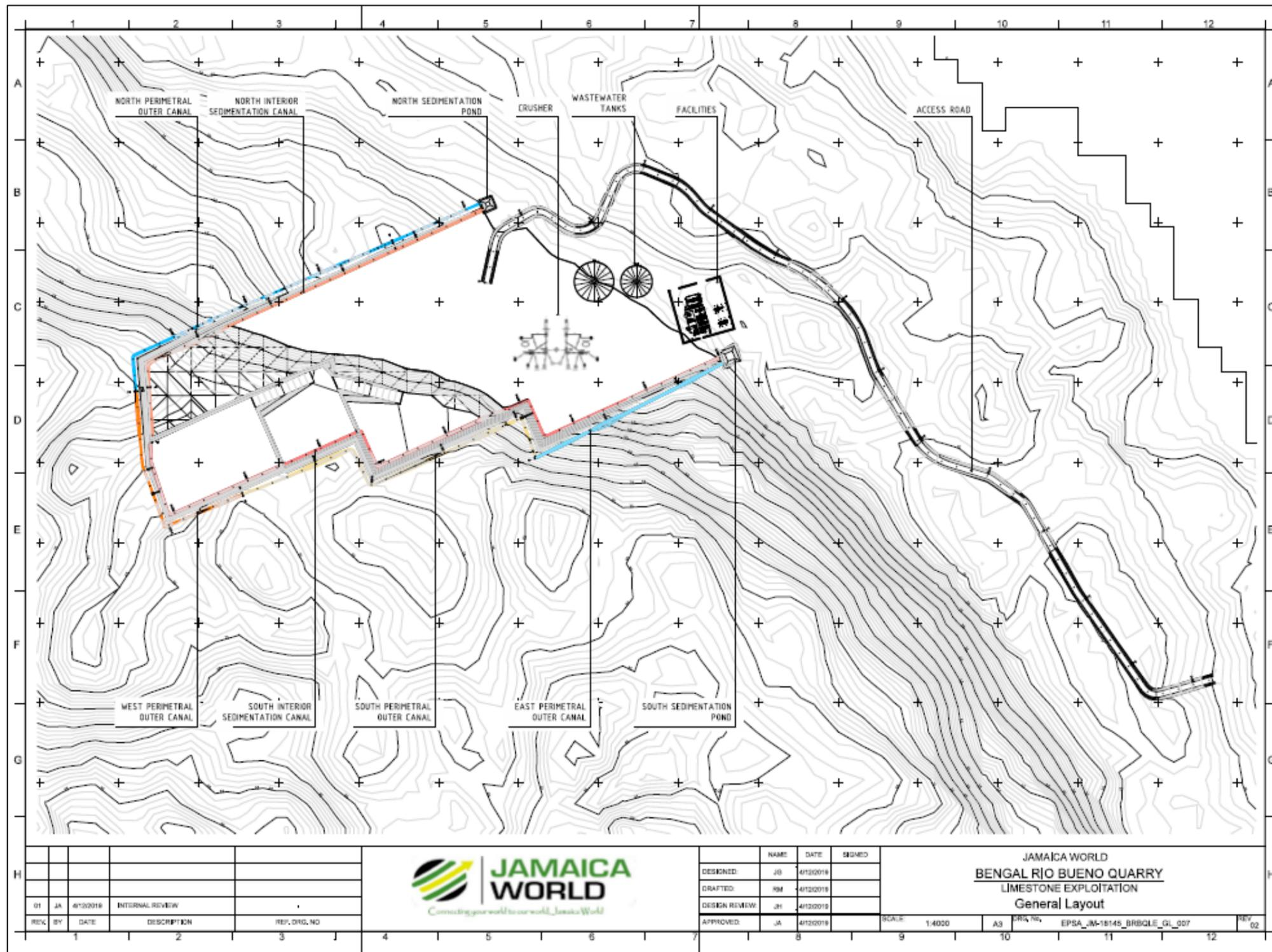
Figure 3-3 General Layout of quarrying facilities on site
