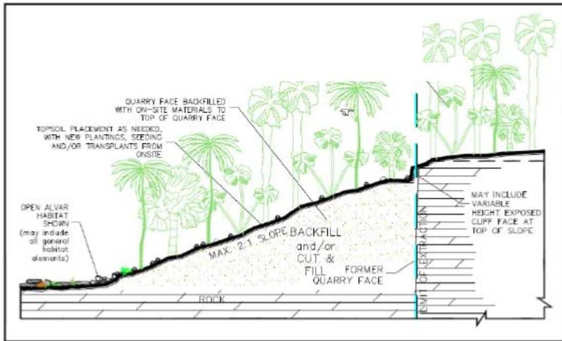
Figure 3-21 Sideslope Detail (backfilled slope)
