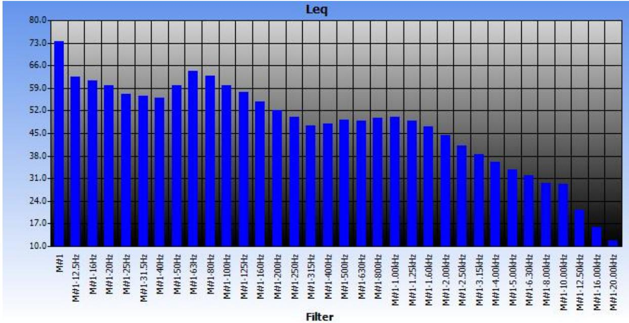
Figure 4-49 Octave band spectrum of noise at Station 9
