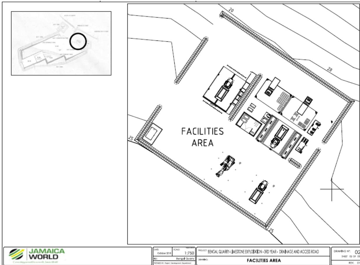
Figure 3-6 Facilities area intended for Contractor’s facilities (workshop, offices and parking area).
