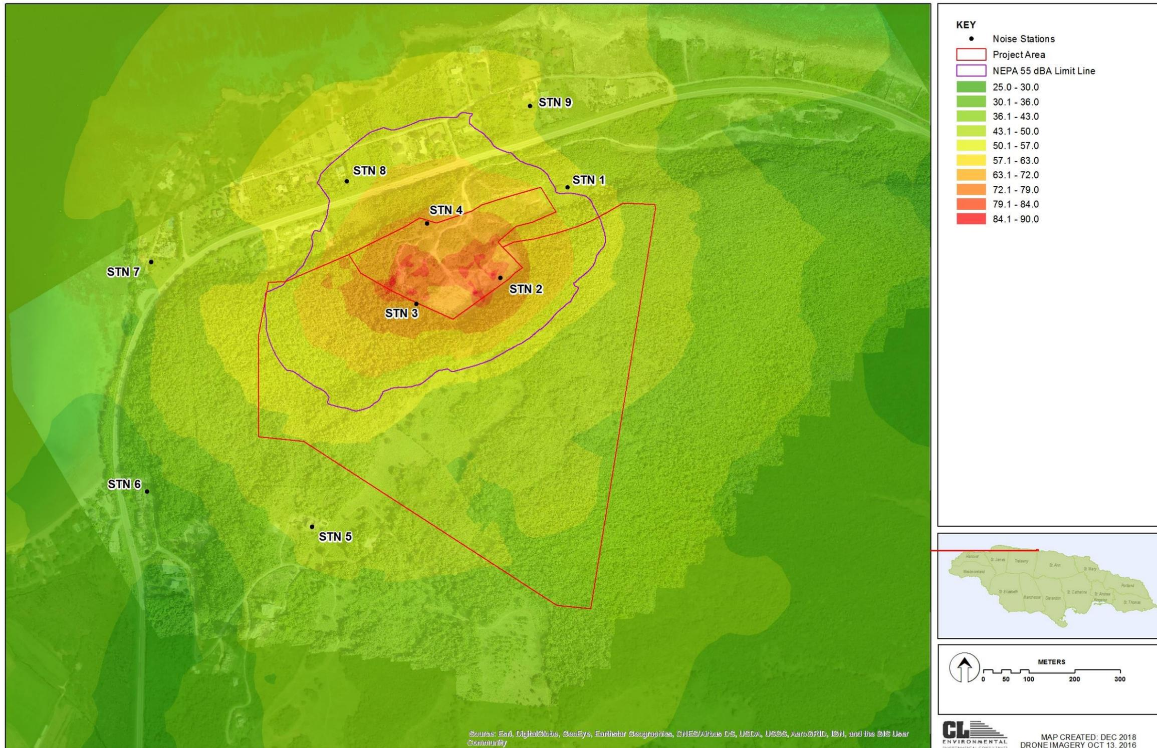
Figure 6-9 Predicted noise emissions from the quarry operations using ISO 9613-2: 1996 Prediction Method
