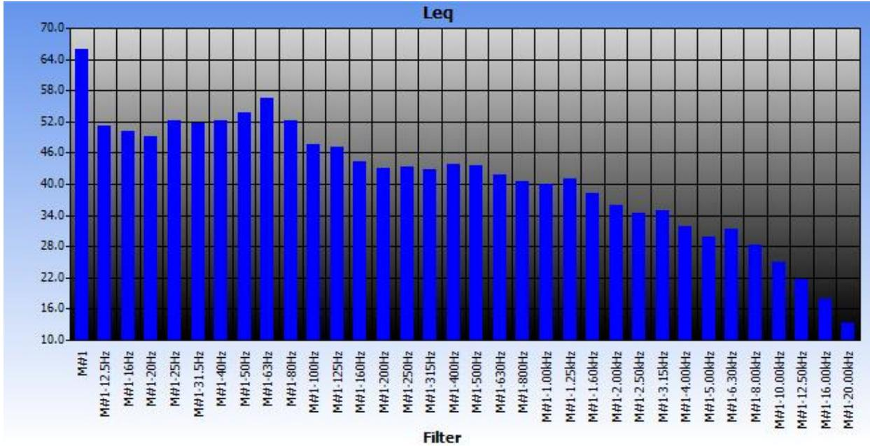
Figure 4-43 Octave band spectrum of noise at Station 7
