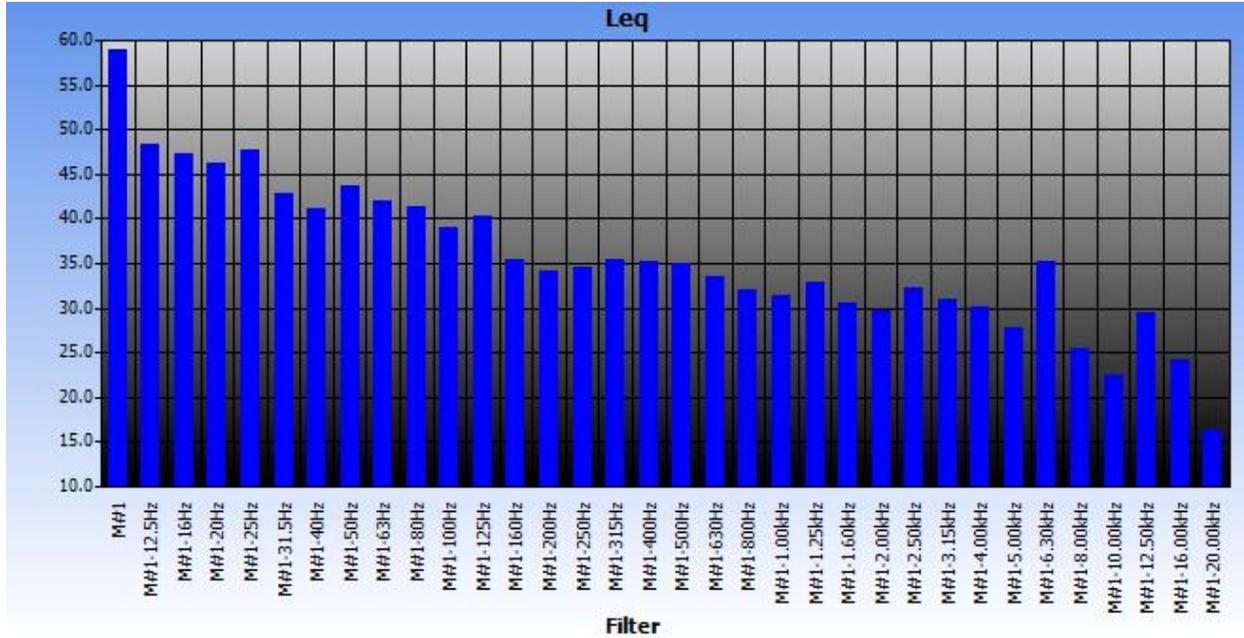
Figure 4-31 Octave band spectrum of noise at Station 3
