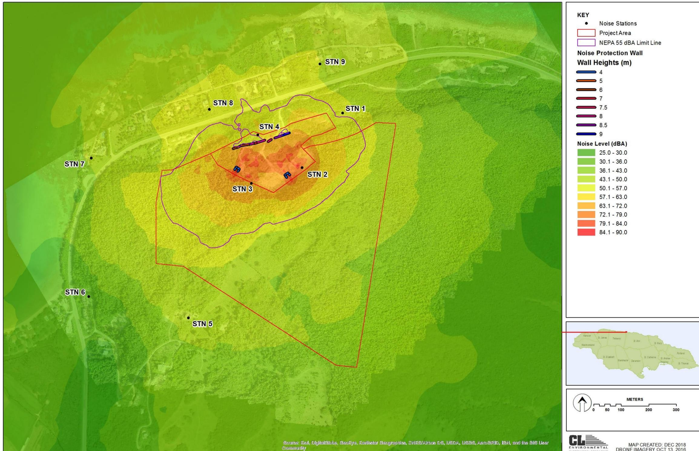
Figure 6-11 Predicted noise emissions from the quarry operations with mitigation using ISO 9613-2: 1996 Prediction Method
