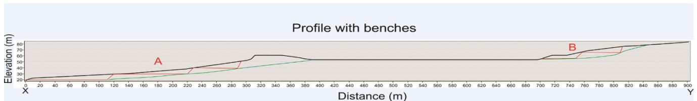
Figure 3-15 Cross section of quarry showing the present topography (black line), bench heights and slope angle (red line) and the target slope angle post-quarrying (green line)
