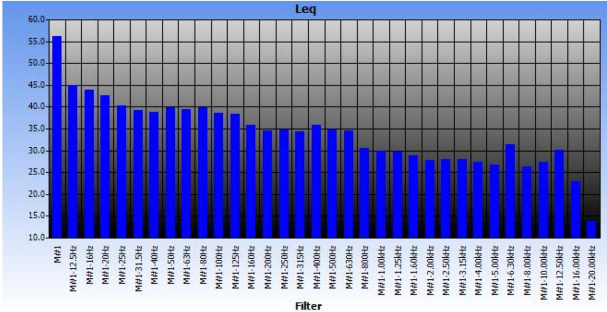
Figure 4-37 Octave band spectrum of noise at Station 5
