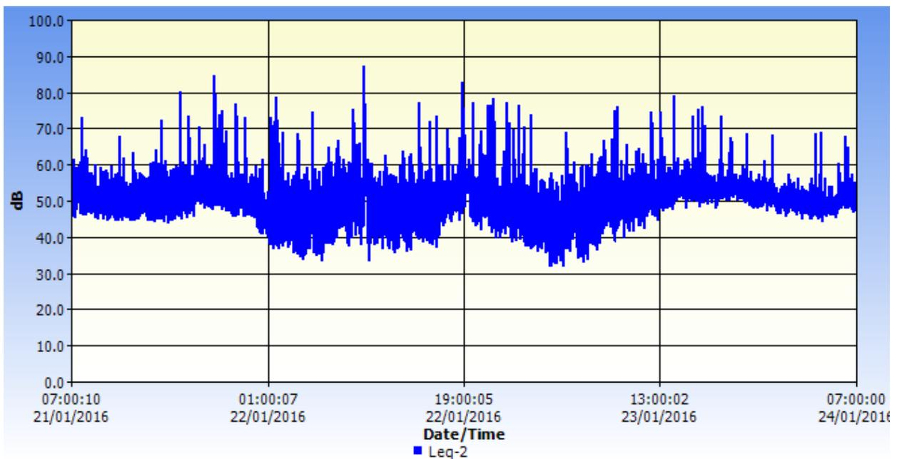
Figure 4-39 Noise fluctuation (Leq) over 72 hours at Station 6
