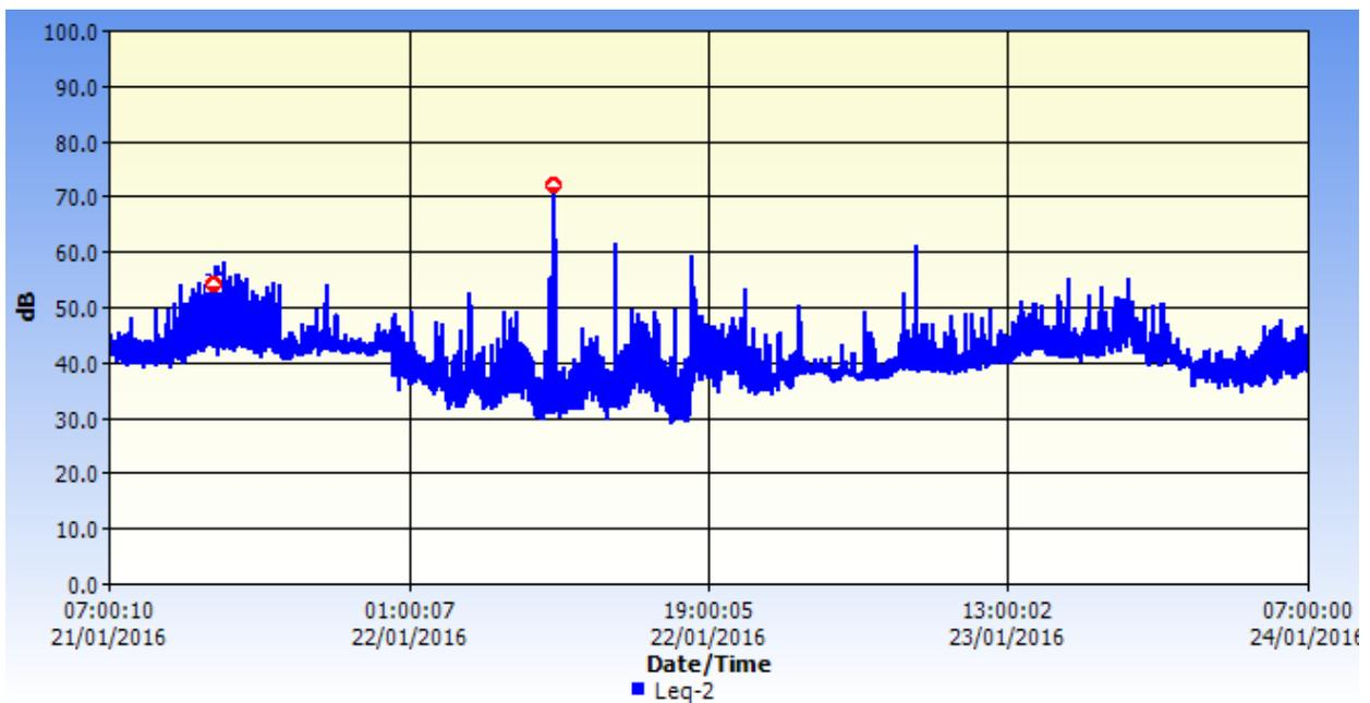
Figure 4-36 Noise fluctuation (Leq) over 72 hours at Station 5
