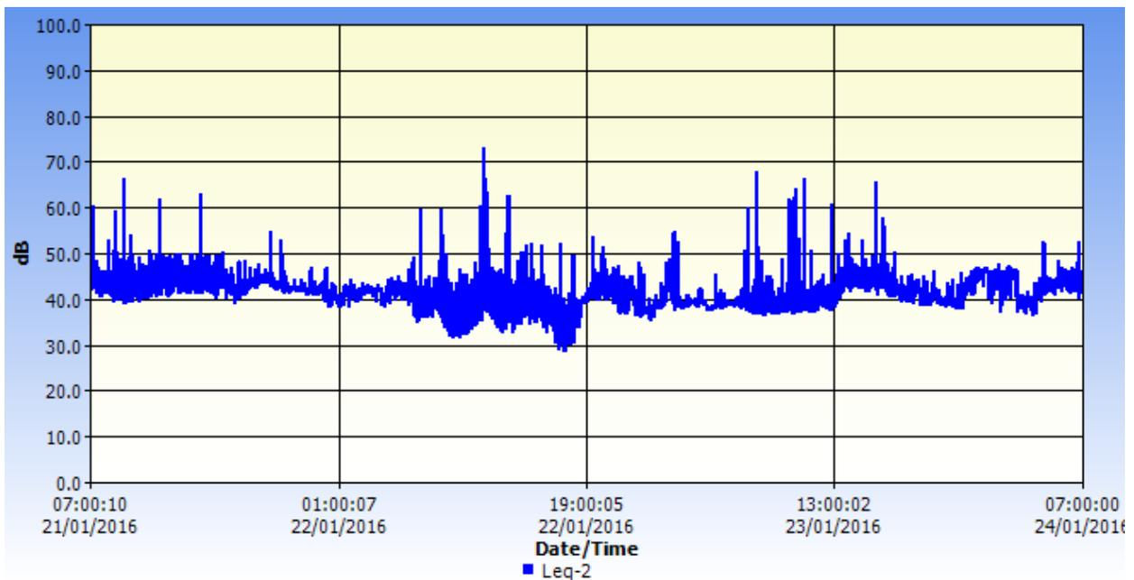
Figure 4-30 Noise fluctuation (Leq) over 72 hours at Station 3
