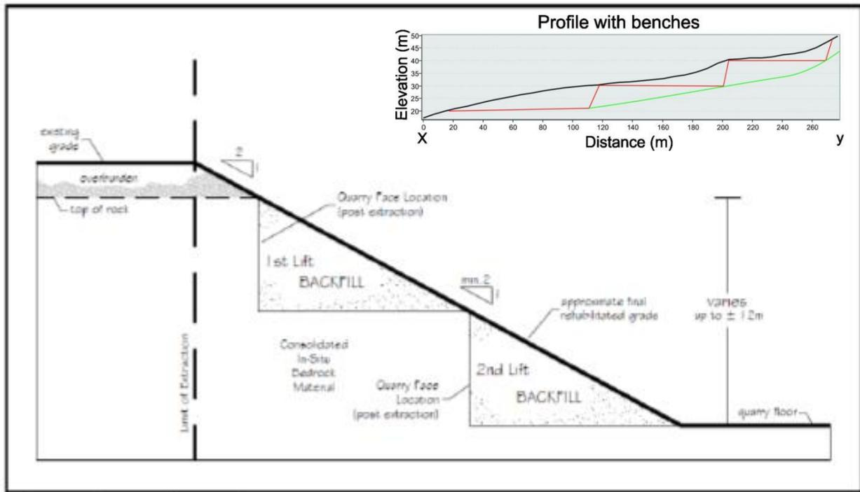
Figure 3-23 Quarry Profile vs Reclaim Slope with Backfill
