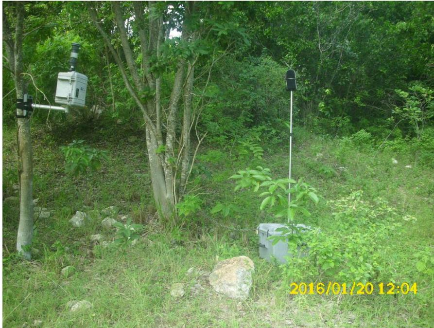
Plate 4-4 Noise (right) and particulate (left) meter
