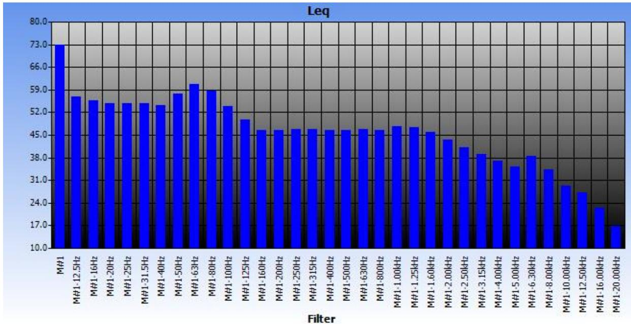
Figure 4-46 Octave band spectrum of noise at Station 8
