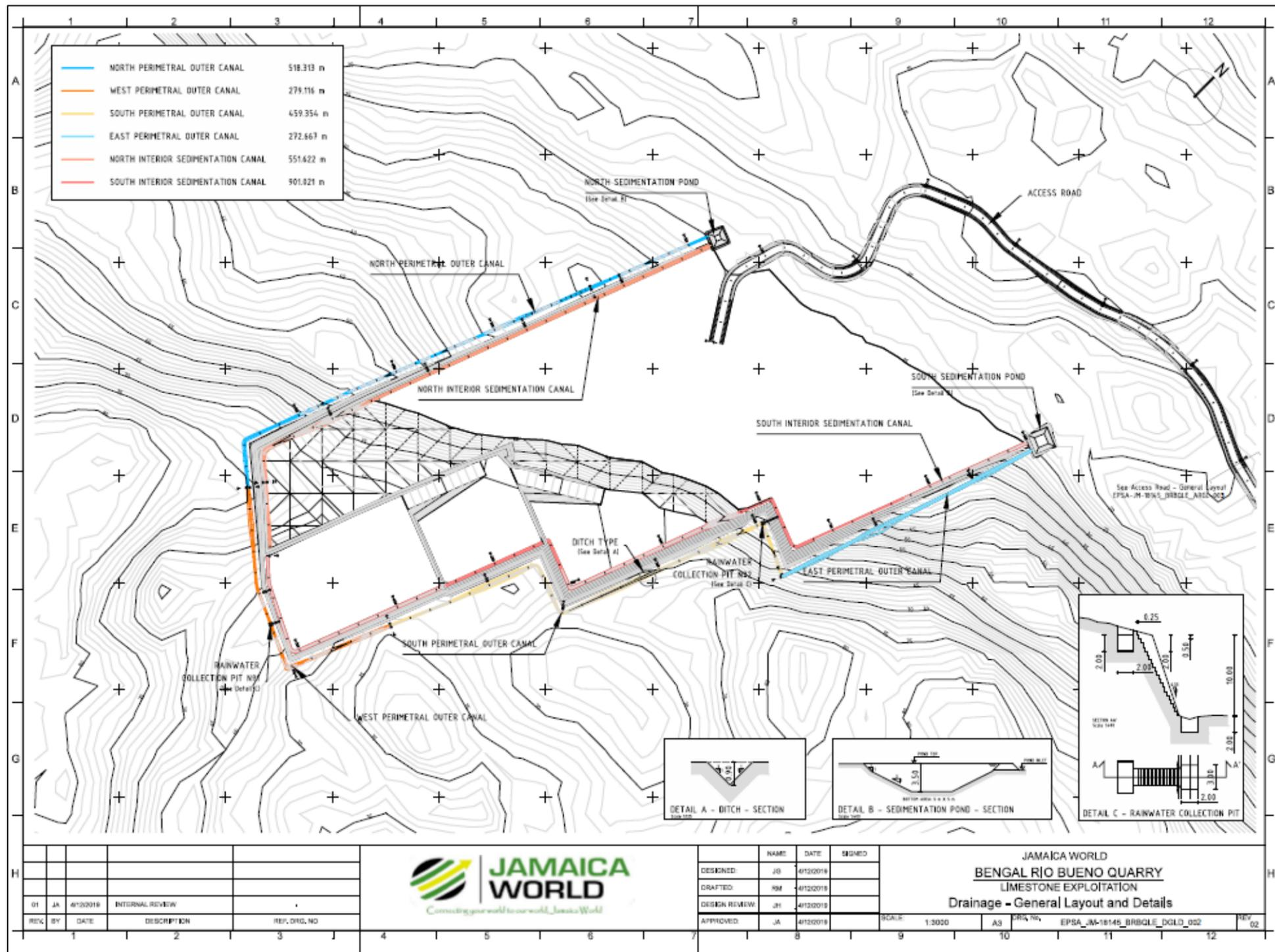
Figure 3-4 Drainage Layout for quarrying facility
