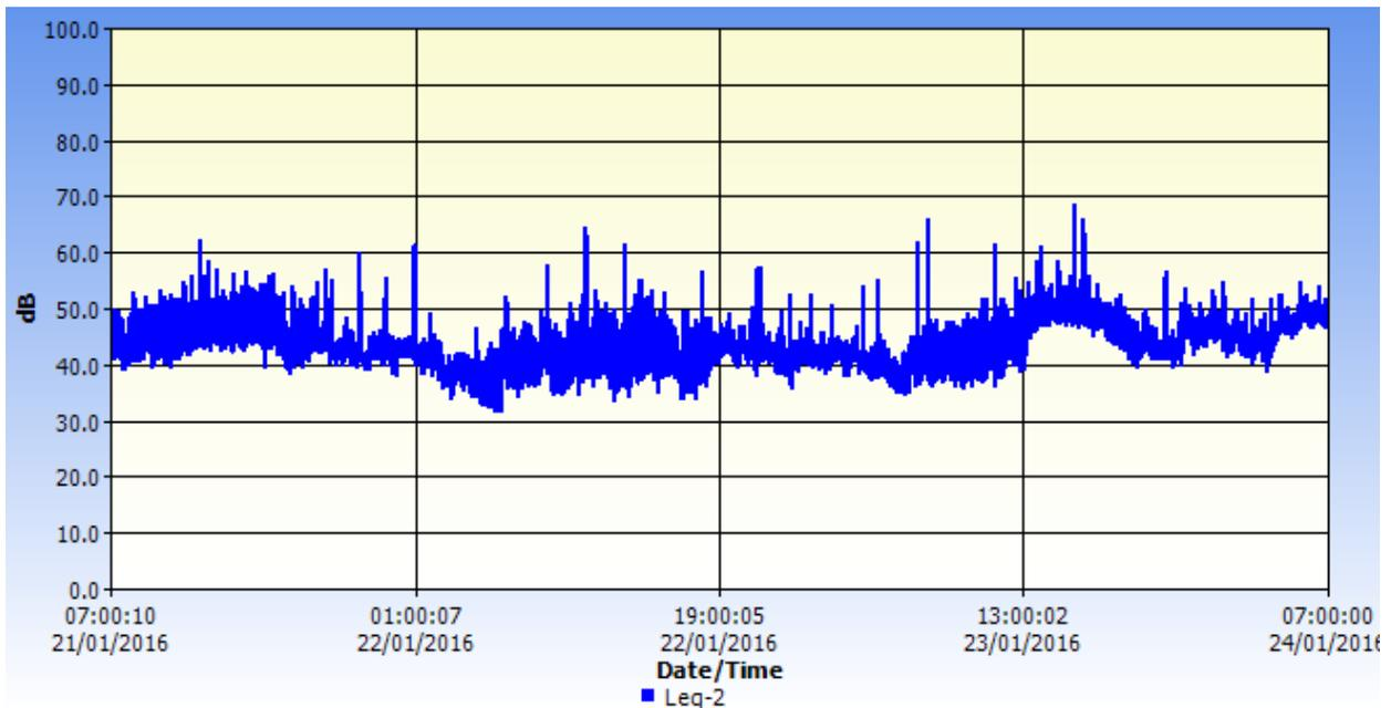
Figure 4-27 Noise fluctuation (Leq) over 72 hours at Station 1
