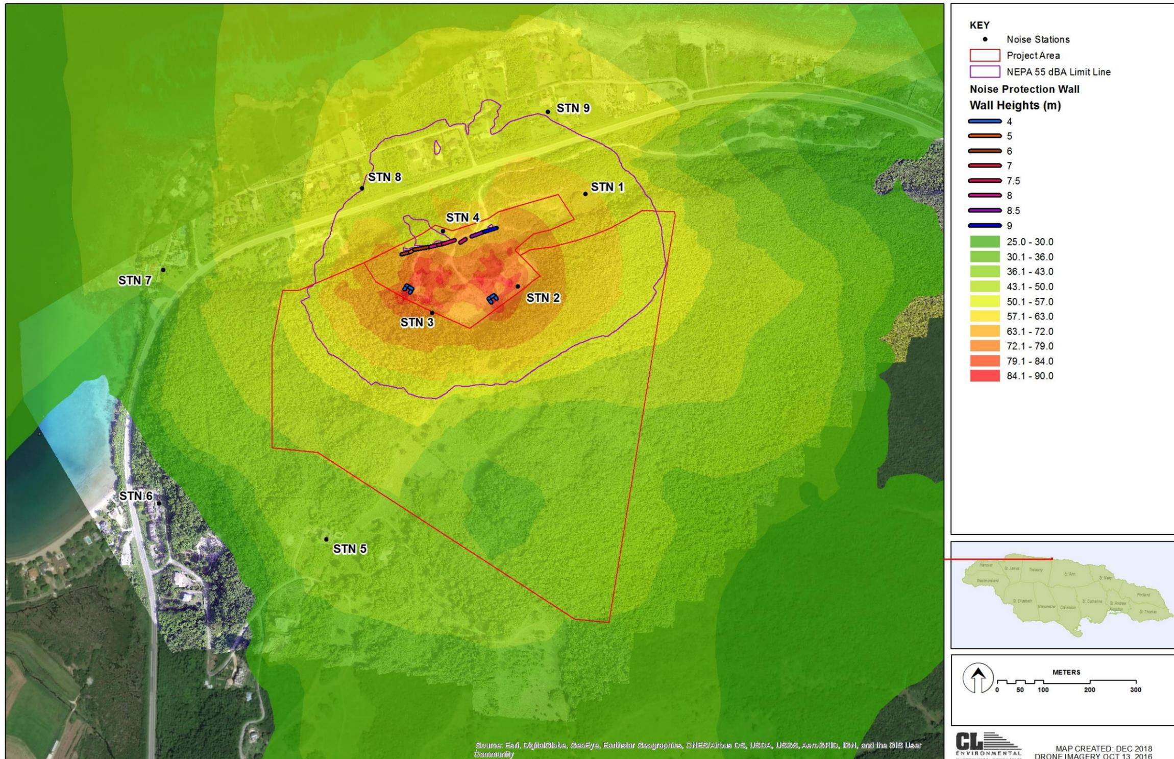
Figure 6-12 Predicted noise emissions from the quarry operations with mitigation using Concawe Prediction Method (wind from the southwest)
