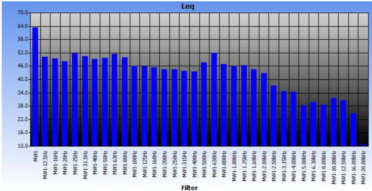
Figure 4-40 Octave band spectrum of noise at Station 6
