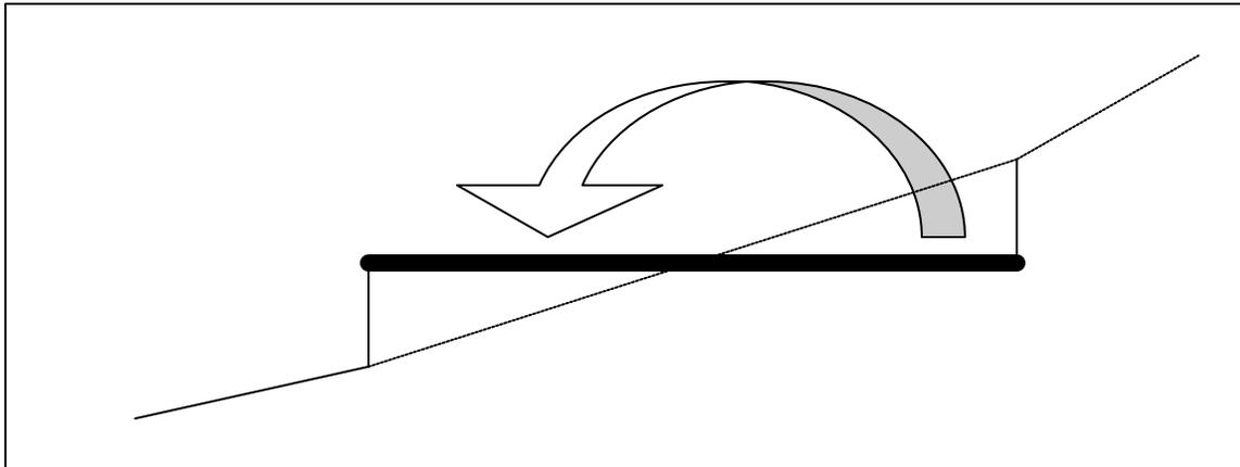
**Figure 4.2 Schematic illustrating cut and fill.**
