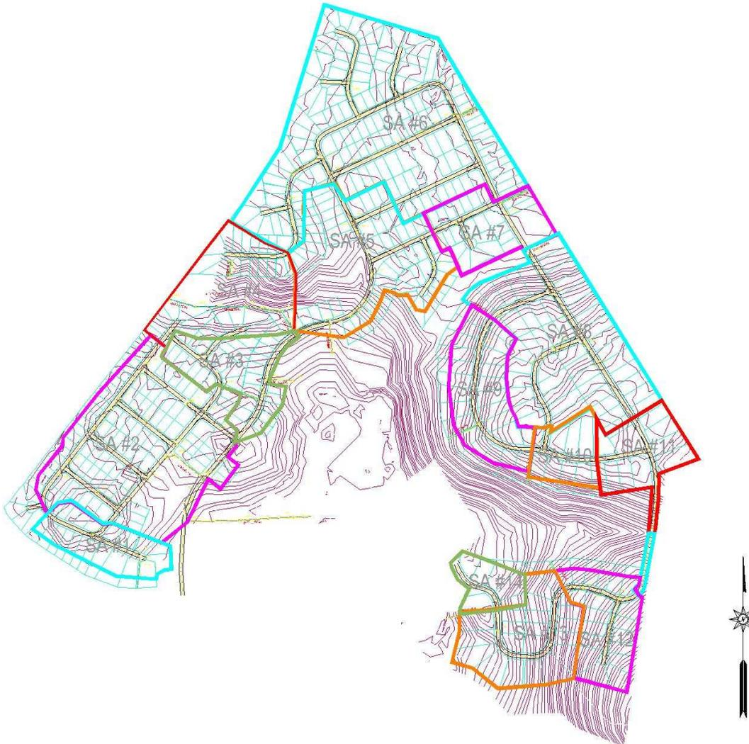
**Figure 6: Internal Drainage Sub-catchments**
