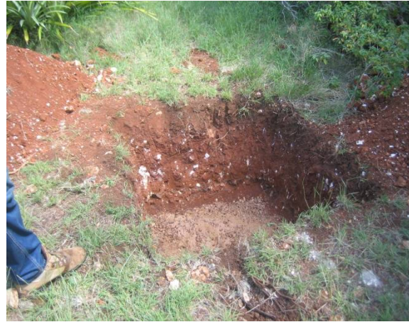
Test pit near marshland reddish brown silty clay intermixed with limestone cobbles and boulders
