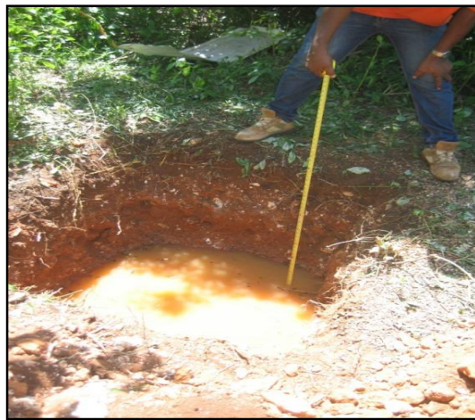
Percolation rate measurement being conducted in Test Pit 3
