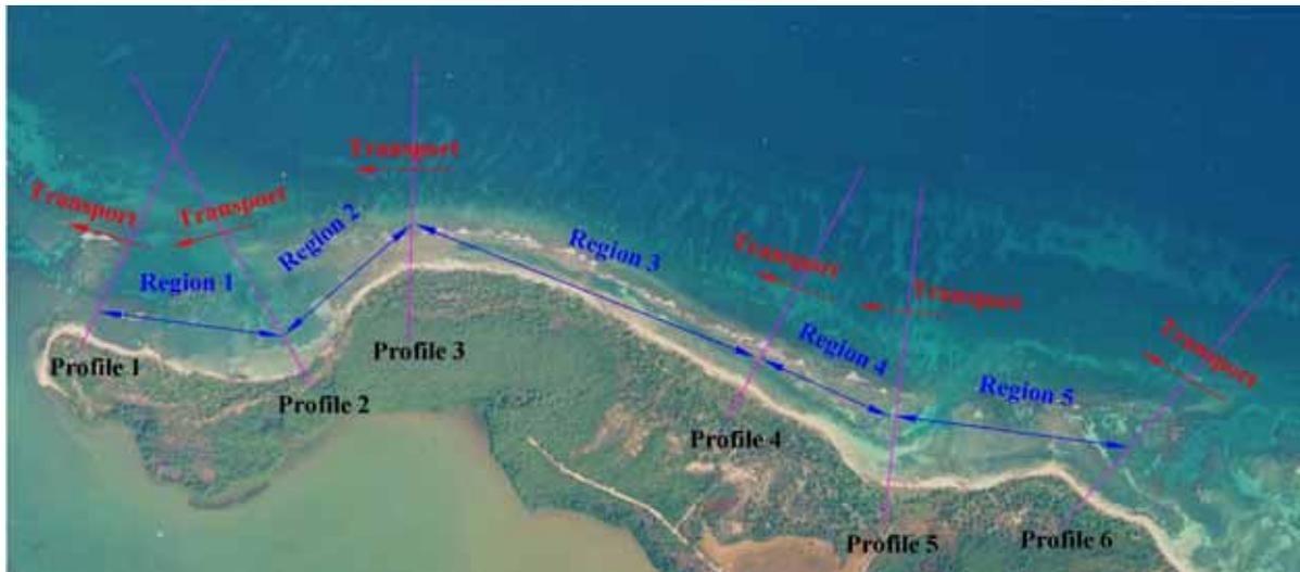
**Figure 4.1 LITPACK Model Profile Lines and Transport Results (arrow lengths indicate relative transport rates)**
