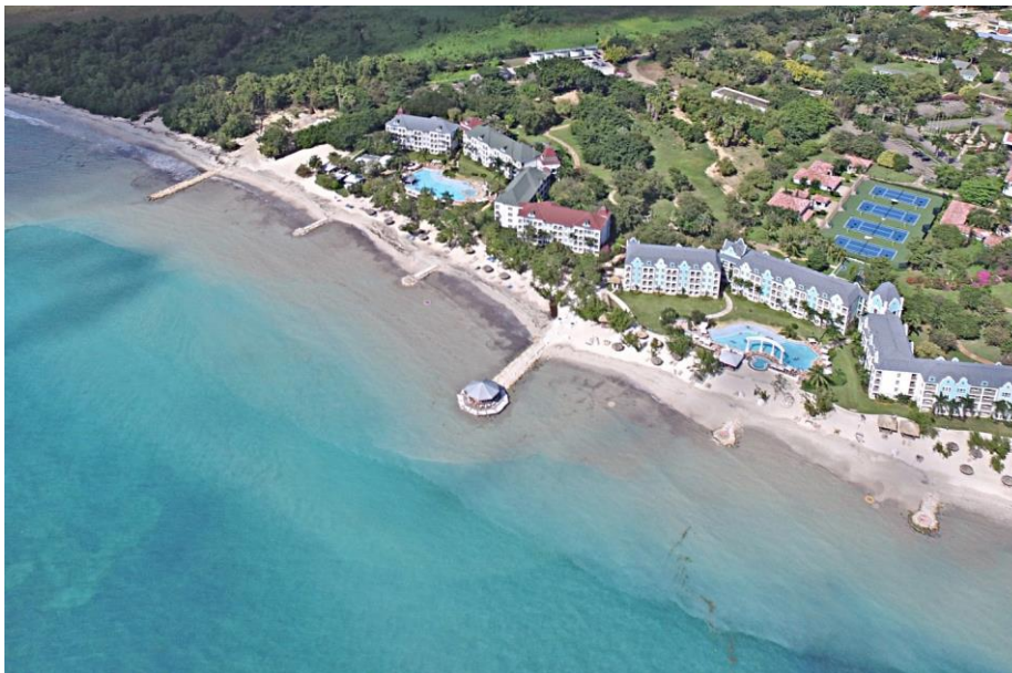
Figure 5.5 Aerial view of groynes placed along French and Dutch Beach segments of the beach. Inshore turbidity following days of rough weather (TEMN 2017 Aerial Photo).
