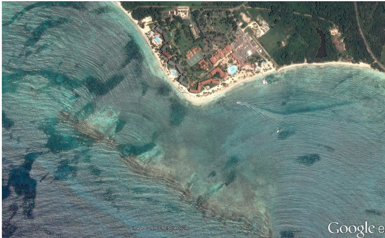
Figure 5.44. Waves converging at the headland due to the diffraction around the ends of the barrier reef results in the wider beach at the tip of the headland.
