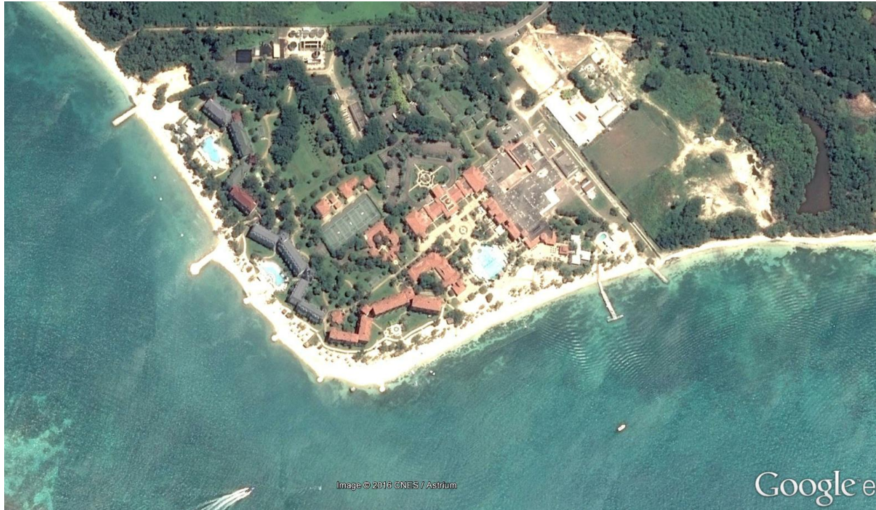
Figure 5.45. Groins around the Sandals Whitehouse headland, note the sand accumulation along the east side of the groin and erosion along the west side.
