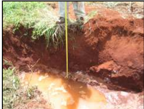
Plate 7: Measurement of percolation rate conducted in test pit.
