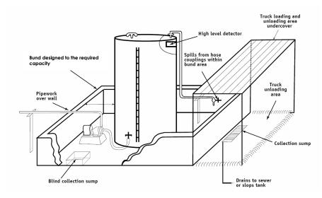
Figure 1 Example of bunding for bulk liquid storage tanks
