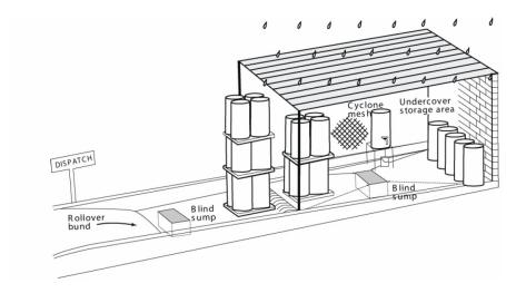
Figure 2 Example of bunding for drums and containers
