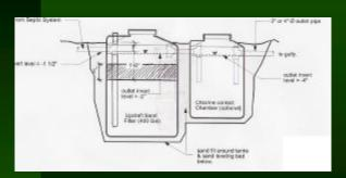
Note: When using a sand filter with some form of disinfection, the final treated effluent will still need to be either reused or disposed of in tile field or soak away pit (these methods are generally preferred over direct discharge into a gully, or river).
