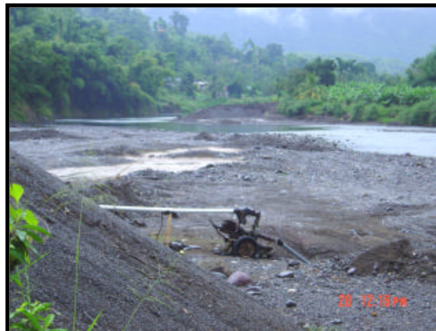
Figure 13. Mining operation at Berridale. To the immediate left, deliberate diversion of the river course to facilitate mining activities is evident.
